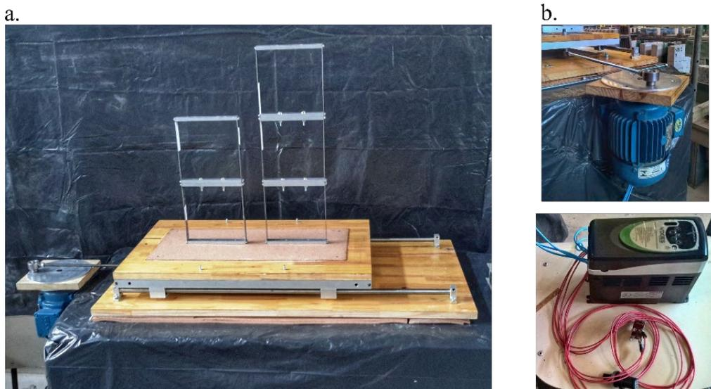
Figure 4. Shaking table built and mechanical and electronic components.
