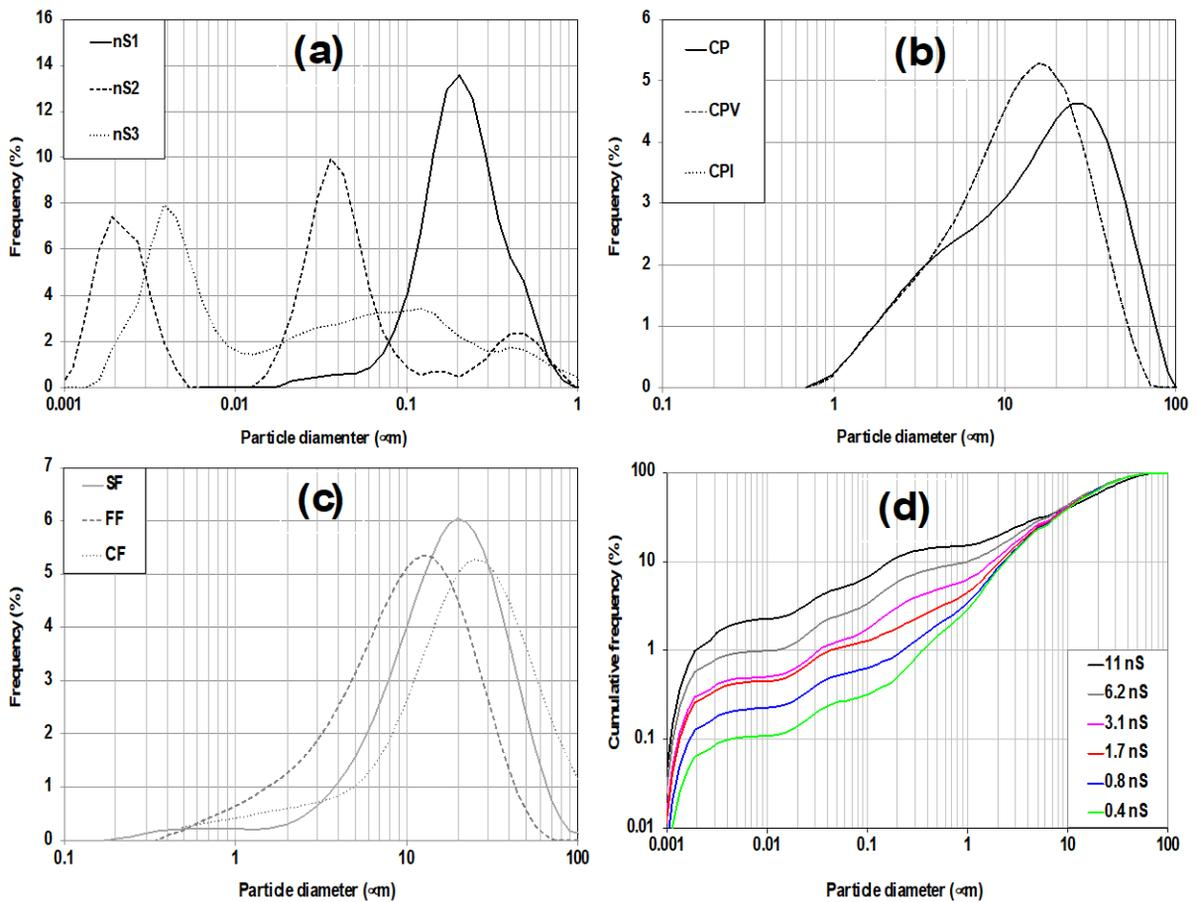
**Figure 3.** Particle size distribution (a) Nano-silicas (b) Cements and Clinker (c) Supplementary Cementitious materials (d) Mixtures
