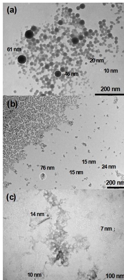
**Figure 2.** Transmission electron micrographies of nano-silicas (a) Cembinder 8 (b) Cembinder 30 and (c) Cembinder 50
