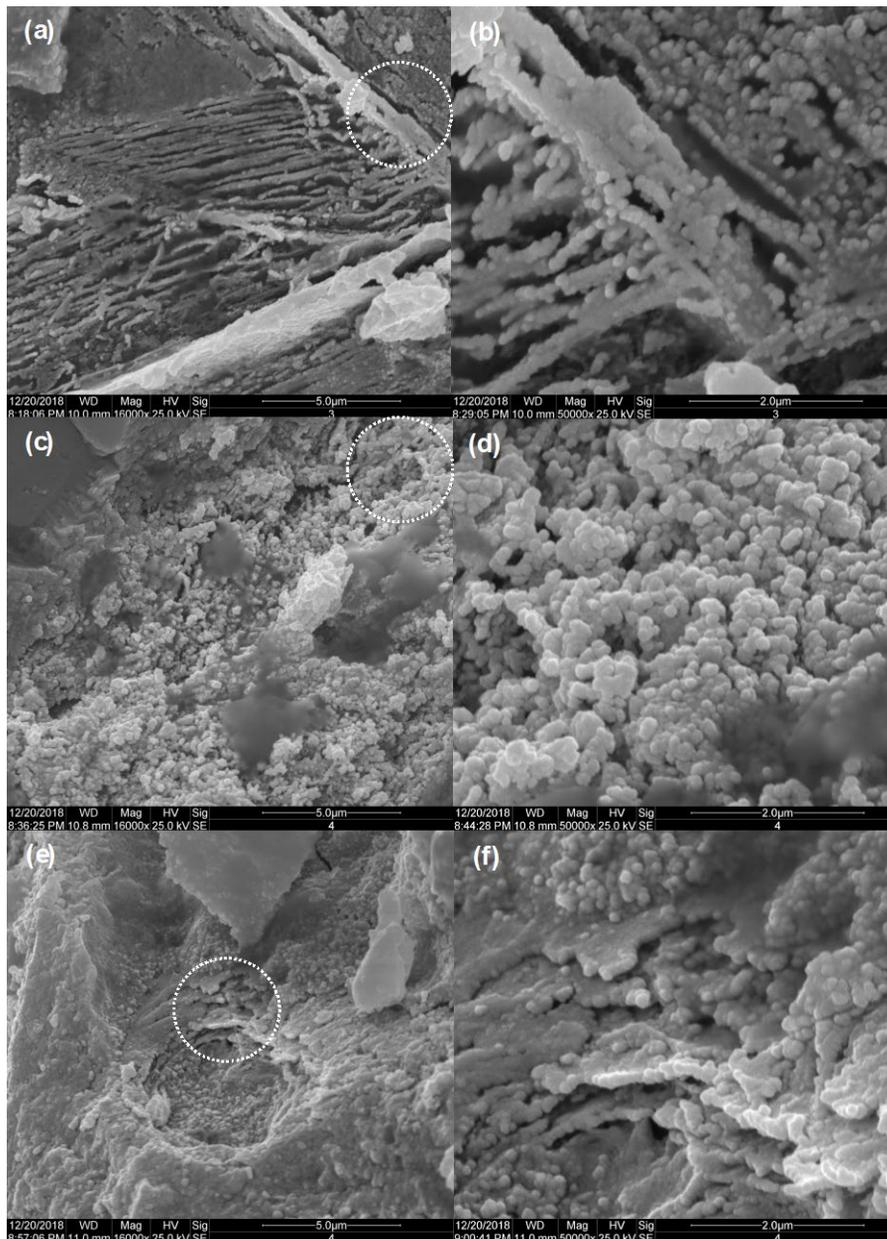
**Figure 7.** SEM micrographics (a, b) CPV-I + SCM + 0.85 nS (c-d) Mixture CP + SCM + 0.85 nS
