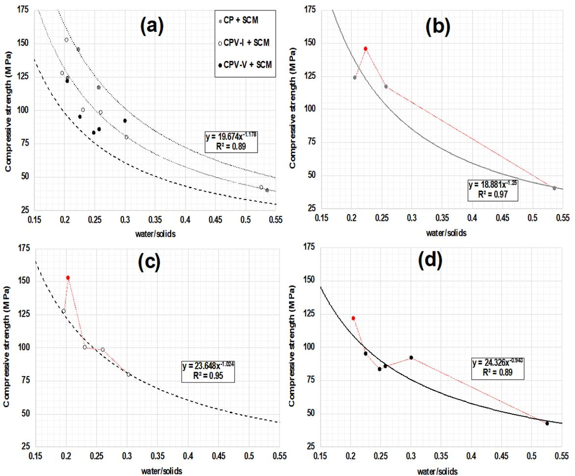
**Figure 5.** Effect of water/solids on the compressive strength (a) all mixtures (b) Pure clinker (c) Portland cement CPV-I (d) Portland cement CPV-V
