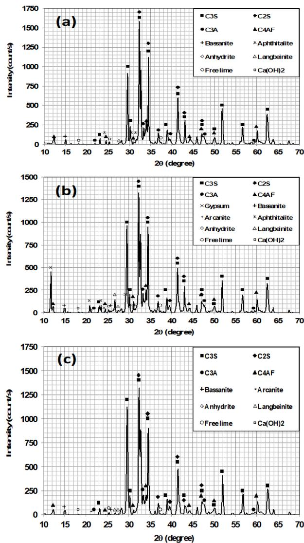
**Figure 1.** Diffractograms (a) Pure Clinker (b) Portland cement CPV-V (c) Portland cement CPV-I. ( $C_3S$ ) -  $3CaOSiO_2$ , ( $C_2S$ ) -  $2CaOSiO_2$ , ( $C_3A$ ) -  $3CaOAl_2O_3$ , ( $C_4AF$ )  $4CaOAl_2O_3Fe_2O_3$ , Gypsum -  $CaSO_4 \cdot 2H_2O$ , Bassanite -  $CaSO_4 \cdot 1/2H_2O$ , Arcanite -  $K_2SO_4$ , Anhydrite -  $CaSO_4$ , Langbeinite -  $K_2Mg_2(SO_4)_3$ , Aphthalite -  $(K, Na)_3Na(SO_4)_2$ , Free lime -  $CaO$  - Portlandite -  $Ca(OH)_2$ . ASTM C1365 [18]
