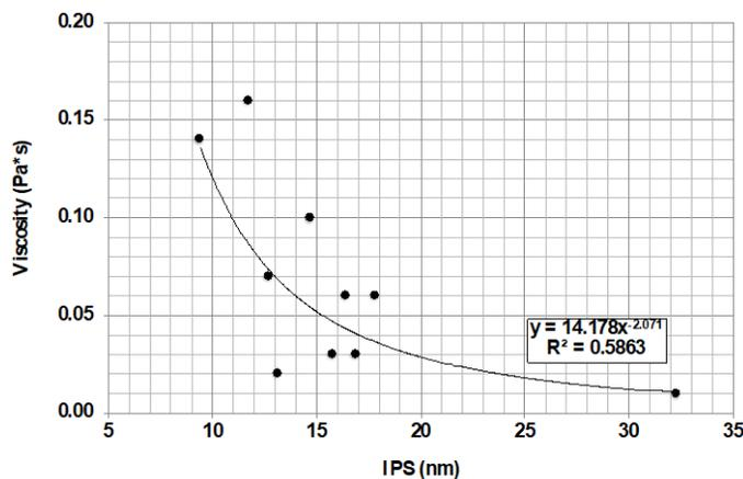
**Figure 4.** Effect of IPS on viscosity of cement pastes
