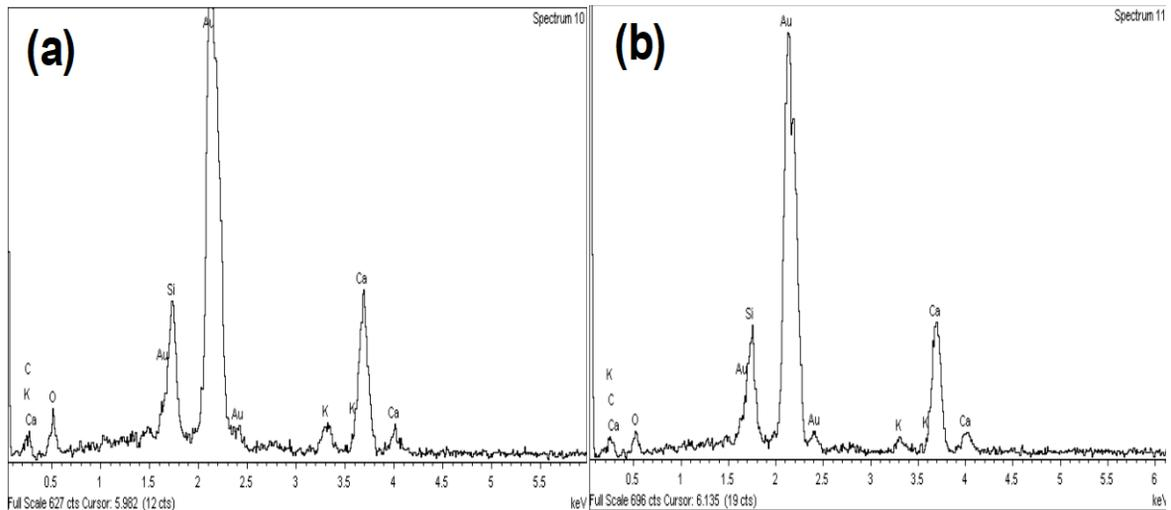
**Figure 8.** Chemical composition obtained by EDS (a) **Figure 7d** and (b) **Figure 7e**
