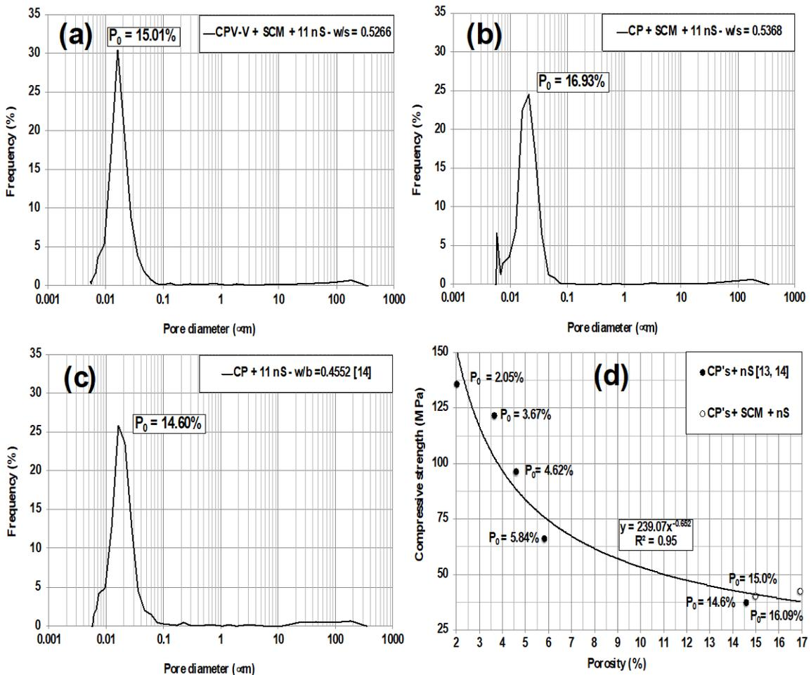
**Figure 6.** Mercury intrusion porosimetry (a) CPV-V + SCM + 11 nS (b) CP + SCM + 11 nS (c) CP + 11 nS and [14] (d) Compressive strength vs Porosity of Portland cement matrices containing nano-silica with and without SCM [13], [14]
