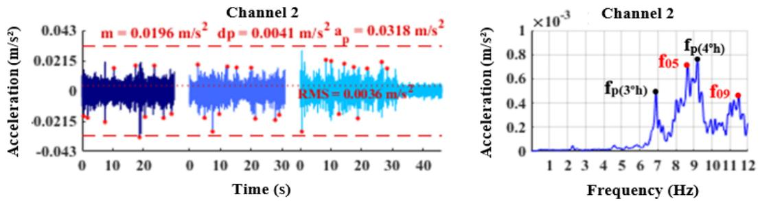
Figure 15. Dynamic response from floor 5 for fast walking on a random trajectory.
