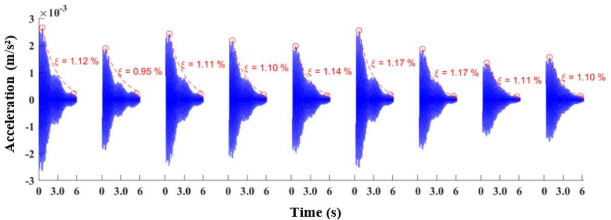
**Figure 9.** Example of the acceleration graph in the time domain filtered at the third mode.
