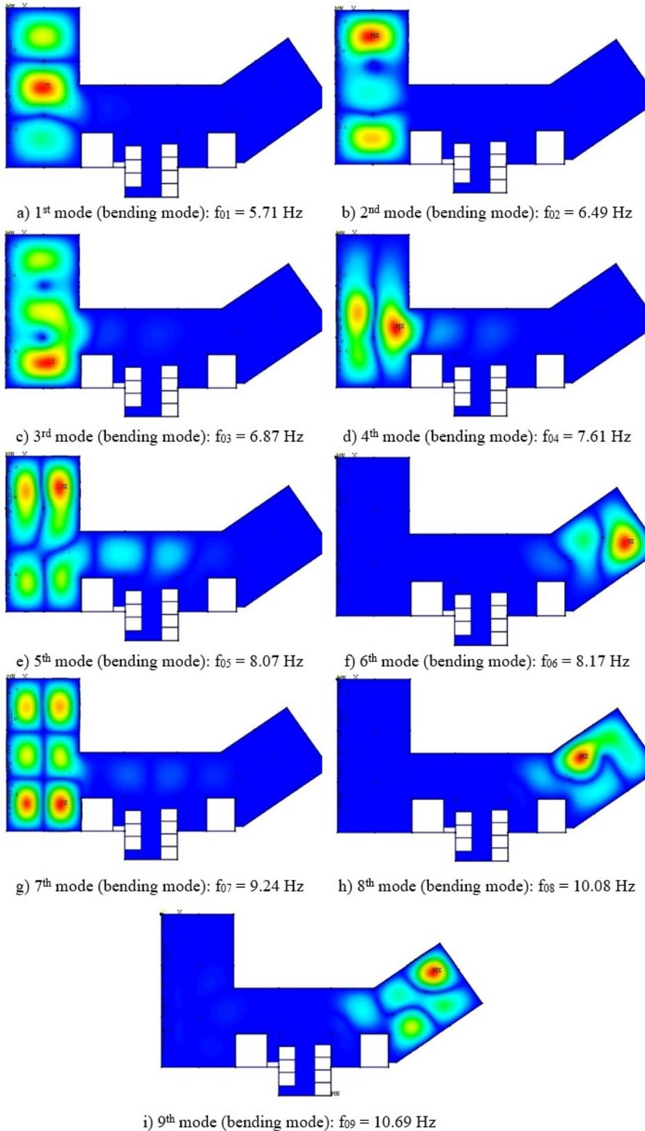
**Figure 10.** Vertical bending vibration modes of the floors under study.
