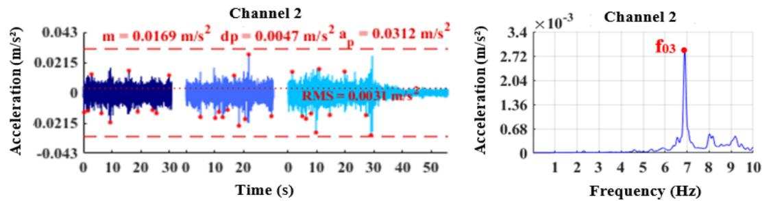
Figure 12. Dynamic response from floor 2 for fast walking on a random trajectory.
