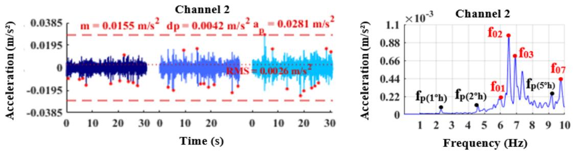
Figure 11. Dynamic response from floor 1 for fast walking on a random trajectory.
