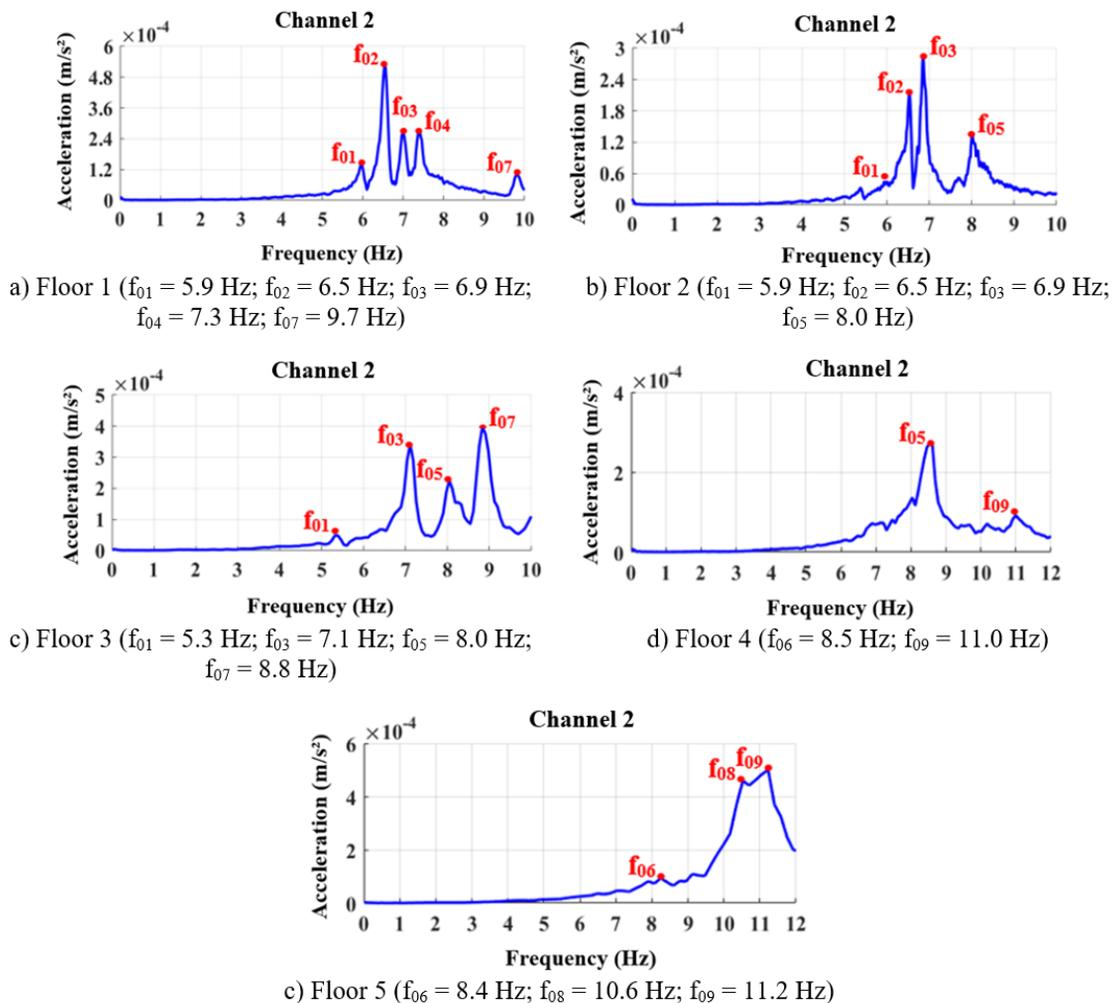
Figure 8. Floor’s vibration modes experimental FFT magnitudes.
