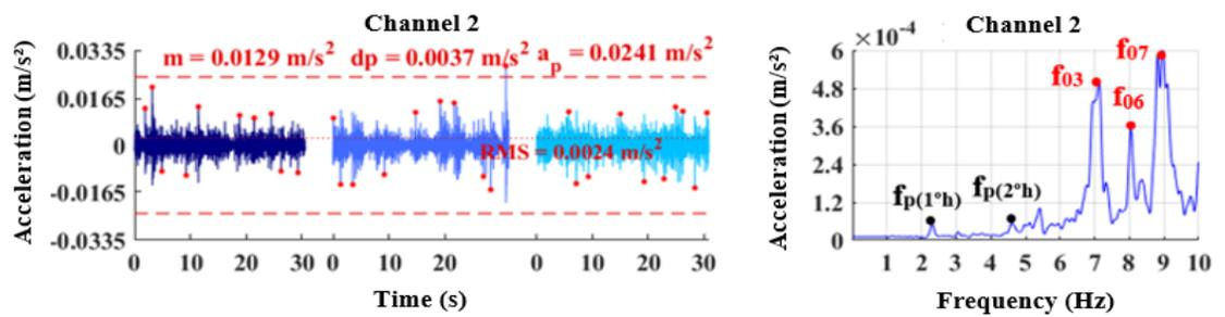
Figure 13. Dynamic response from floor 3 for fast walking on a random trajectory.
