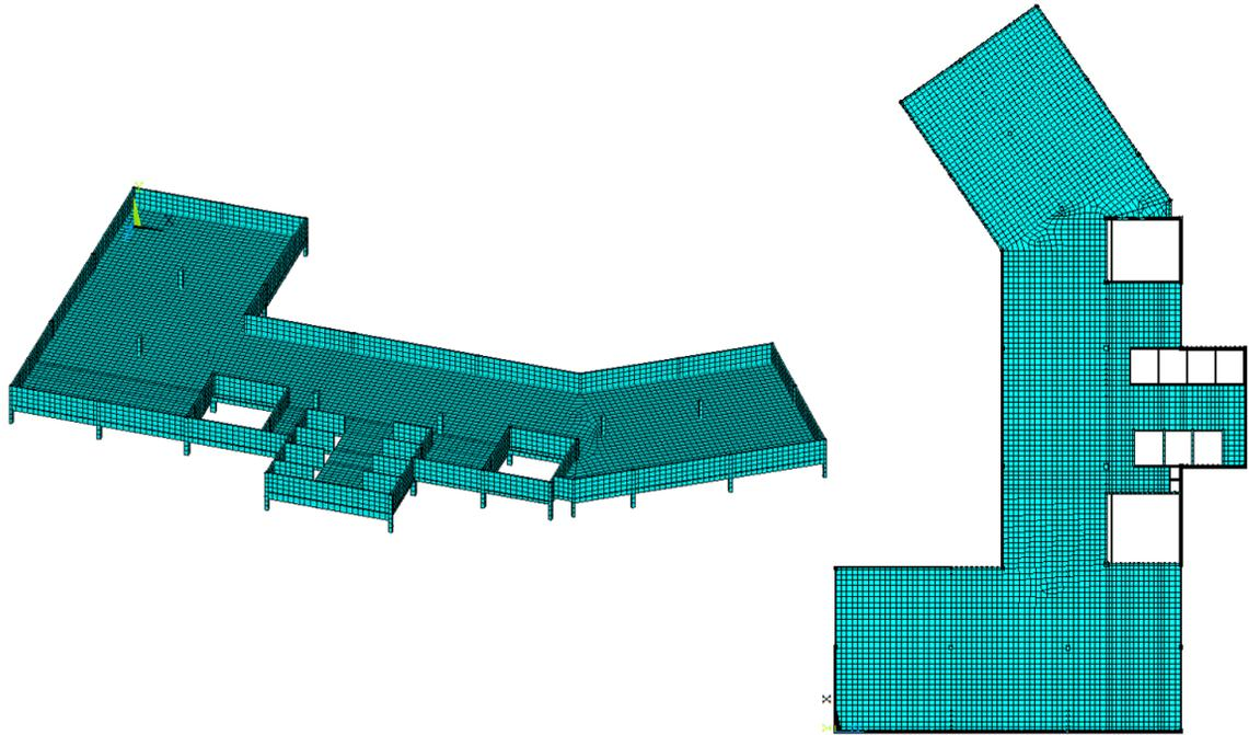
**Figure 4.** Investigated composite floor (steel-concrete) finite element model.
