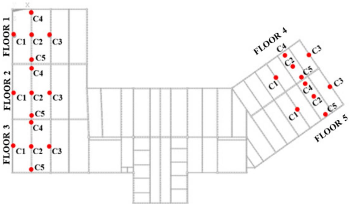
Figure 5. Instrumentation points over the five tested floors.
