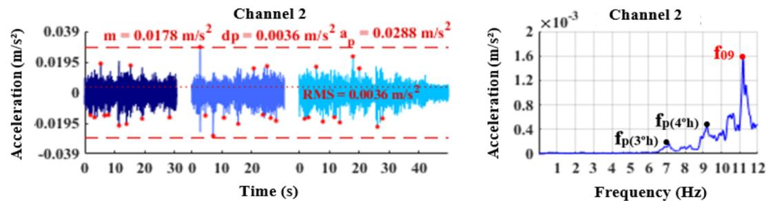
Figure 14. Dynamic response from floor 4 for fast walking on a random trajectory.
