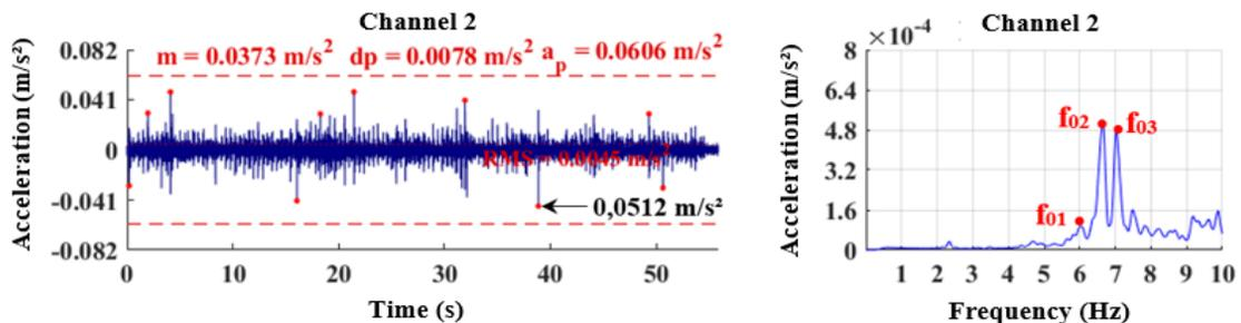
Figure 16. Dynamic response from floor 1 for four fast walking people on a random trajectory.
