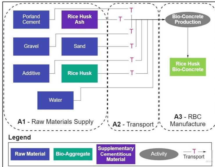
Figure 2. System boundaries for the production of Rice husk bio-concrete.
