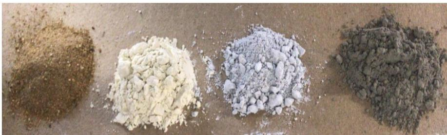
**Figure 1.** From left to right: fine aggregate, glass powder, silica fume, and cement.
