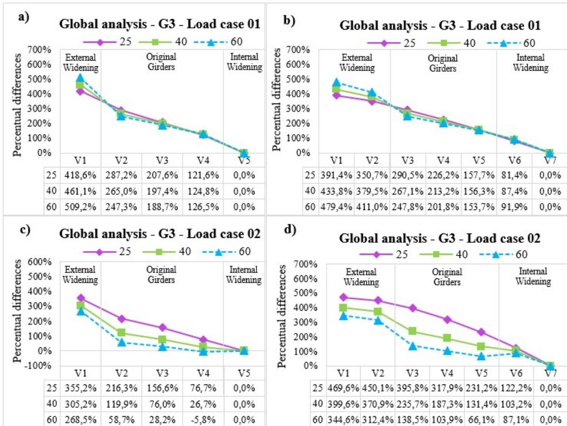
**Figure 11.** Global analysis of the BMDF's for the models with 25, 40, and 60 MPa widening, in comparison to the innermost girder: (a) 5L-G3 (Load case 01); (b) 7L-G3 (Load case 01); (c) 5L-G3 (Load case 02); (d) 7L-G3 (Load case 02).
