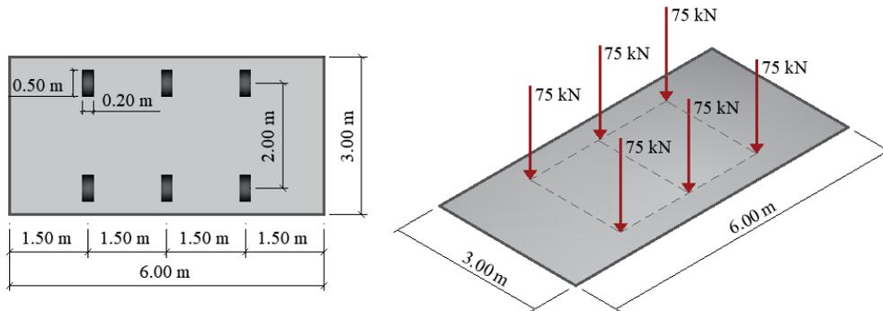
Figure 5. Vehicle type TB-450. Adapted from ABNT NBR 7188 [15].
