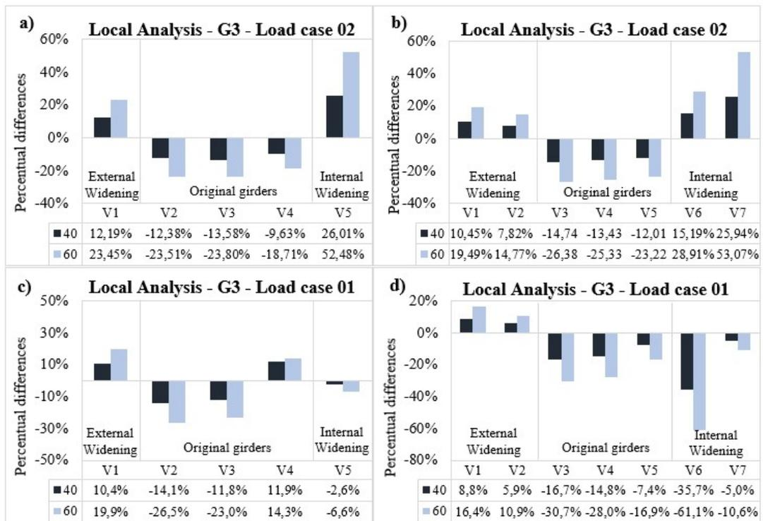
**Figure 12.** Local analysis of the BMDF's for models with 40 and 60 MPa widening, compared to the models with uniform stiffness.: (a) 5L-G3 (Load case 02); (b) 7L-G3 (Load case 02); (c) 5L-G3 (Load case 01); (d) 7L-G3 (Load case 01).
