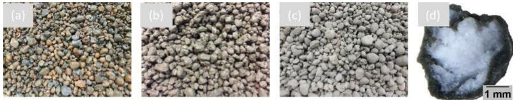
Figure 4 - Before and after cement coating application on substitute aggregate capsules for EC (a, b) and EP (c, d)
