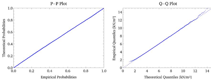
**Figure 6.** P-P and Q-Q probability plots showing the deviation of  $L_{50}$  from the fitted Gumbel distribution in an office floor with  $A = 100 \text{ m}^2$ .
