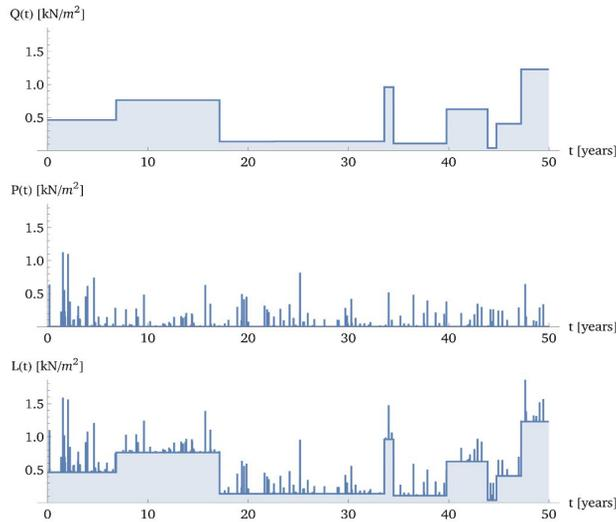
Figure 3. Time histories of one sample of sustained, extraordinary and total live load for an office floor with  $A = 500 \text{ m}^2$ .
