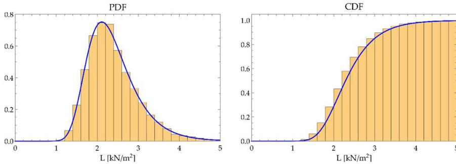
**Figure 5.** Probability density and cumulative distribution histograms vs. fitted Gumbel distribution for  $L_{50}$  in an office floor with  $A = 100 \text{ m}^2$ .
