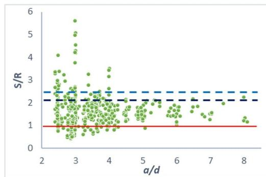
Figure 13- S/R in relation to  $a/d$  to NBR 6118:2014
