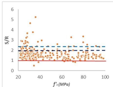
**Figure 8-** S/R in relation to  $f'_c$  to Frosch et al. [5]
