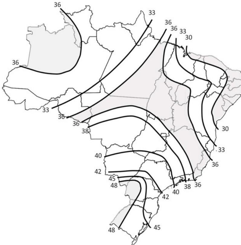
**Figure 22.** Final basic wind speed map proposed for NBR 6123 (isopleths with  $V_0$  in m/s).
