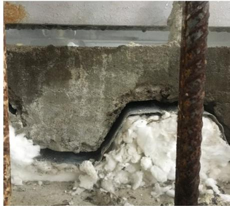
Figure 7 – Detachment of the steel decking during test
