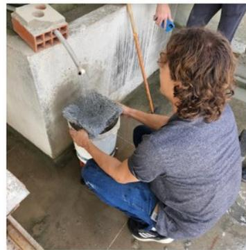
(b) Flow coefficient test.
