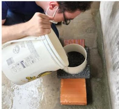
(a) Permeability coefficient test
