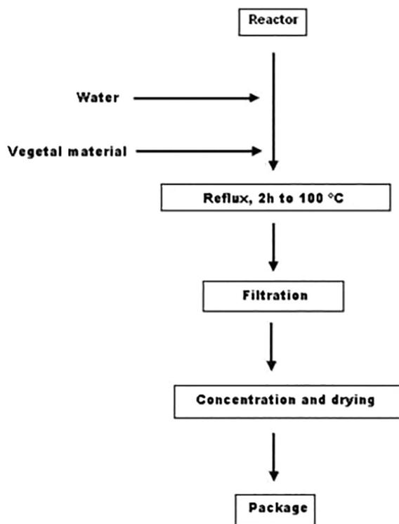
FIGURE 1 - Technological process diagram.
