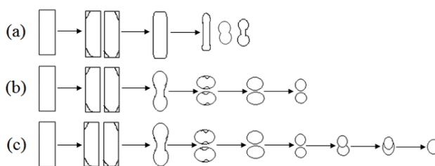
FIGURE 7 - The probable formation mechanisms of pellets in spheronization process(a) clavate, double sphere or dumb-bell shaped pellets; (b) spherical pellets;(c) oversized pellets.
