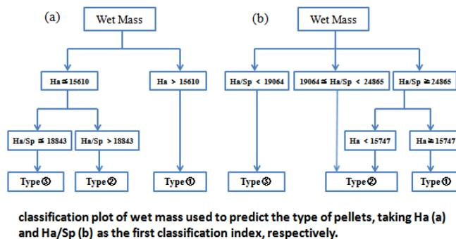
FIGURE 6 - classification plot of wet mass used to predict the type of pellets, taking Ha (a) and Ha/Sp (b) as the first classification index, respectively.
