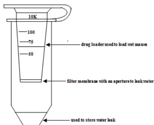
**FIGURE 1** - The schematic diagram of ultrafiltration centrifuge tube.
