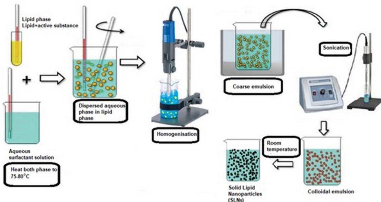
**FIGURE 1** - Preparation of SLNs with homogenization/sonication method.
