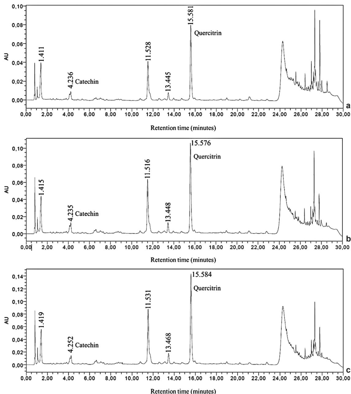
**Figure 1** – a-c. Chromatographic profile obtained by UHPLC-UV- DAD, in  $\lambda = 270$  nm, for EtOH *C. lineatifolia* extract, in different extractive methods – a. extract EtOH UB; b. extract EtOH ES; c. extract EtOH R. Legend: UHPLC-UV- DAD = ultra-high performance liquid chromatography coupled to ultraviolet-photodiode array detector; EtOH = ethanol; UB = maceration under ultrasonic bath; ES = maceration under electromagnetic stirring; R = extraction in continuous reflux system.
