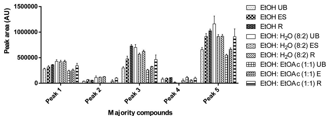
**Figure 2** – Peak areas of the major compounds (peaks 1 to 5) of *C. lineatifolia* extracts obtained by UHPLC-UV-DAD in different extractive methods and solvents. Each bar represents the mean  $\pm$  SEM, Two-way ANOVA, with Tukey's post-test comparison ( $n = 3$ ),  $p < 0.05$ . Legend: EtOH = ethanol; H<sub>2</sub>O = water; EtOAc = ethyl acetate; UB = maceration under ultrasonic bath; ES = maceration under electromagnetic stirring; R = extraction in continuous reflux system.
