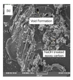
Figure 11. Scanning electron microscopy images of composites (a) processed and (b) unprocessed tensile results.
