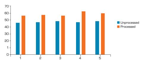
Figure 2. Tensile strength vs. composite process comparison.
