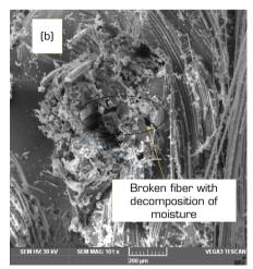
Figure 13. Scanning electron microscopy images of composites (a) processed and (b) unprocessed shear load.
