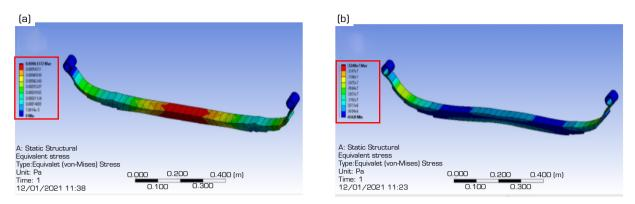
Figure 8. Composite finite element analysis impact plot results for (a) deformation and (b) flexural stress.
