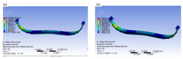
Figure 6. Composite finite element analysis simulation plot results for (a) deformation and (b) flexural stress
