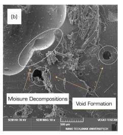
Figure 12. Scanning electron microscopy images of composites (a) processed and (b) unprocessed flexural load.
