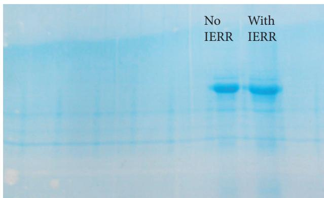
**Figure 4** - 12% SDS-PAGE gel for the GCF of patients with and without IERR obtained by means of the new extraction method.
