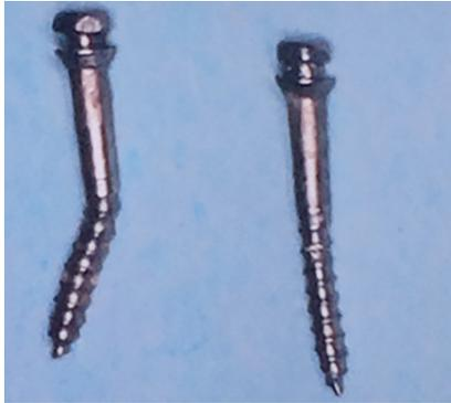
**Figure 5** - Force application too far from bone/microimplant interface, resulting in MI deformation.
