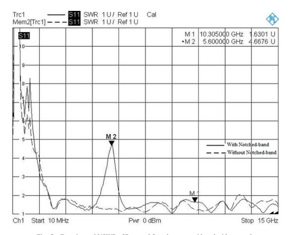
Fig. 7. Experimental VSWR of Proposed fractal antenna with and without notch
