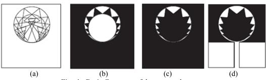
Fig. 1. Basic Geometry of the proposed antenna
