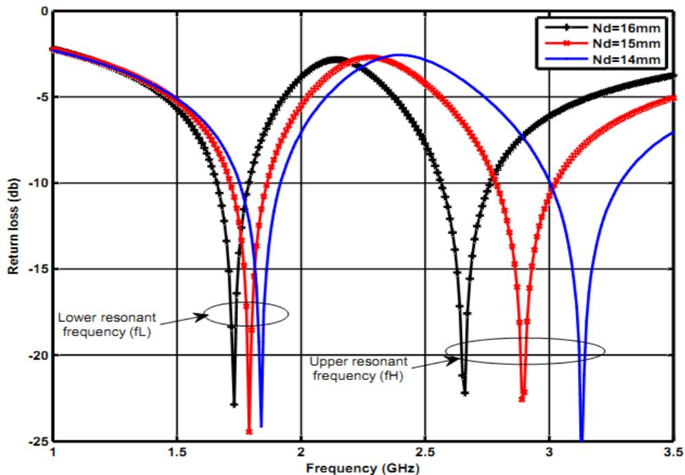
Fig.4 Variation of return loss with frequency for different notch depth ( $N_d$ )
