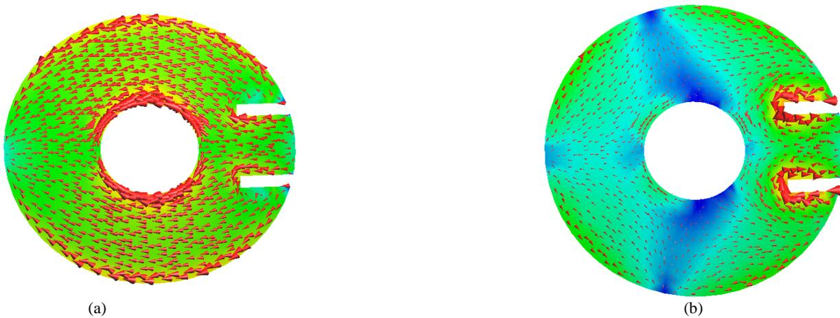
**Fig.3** Current distribution on the patch at (a) 1.5 GHz (b) 2.68 GHz
