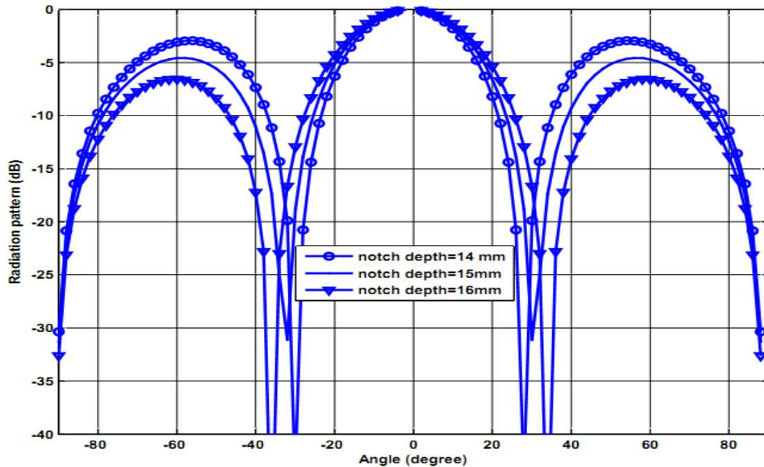
Fig. 9 Variation of radiation pattern at upper resonance frequency for different values of notch depth ( $N_d$ )
