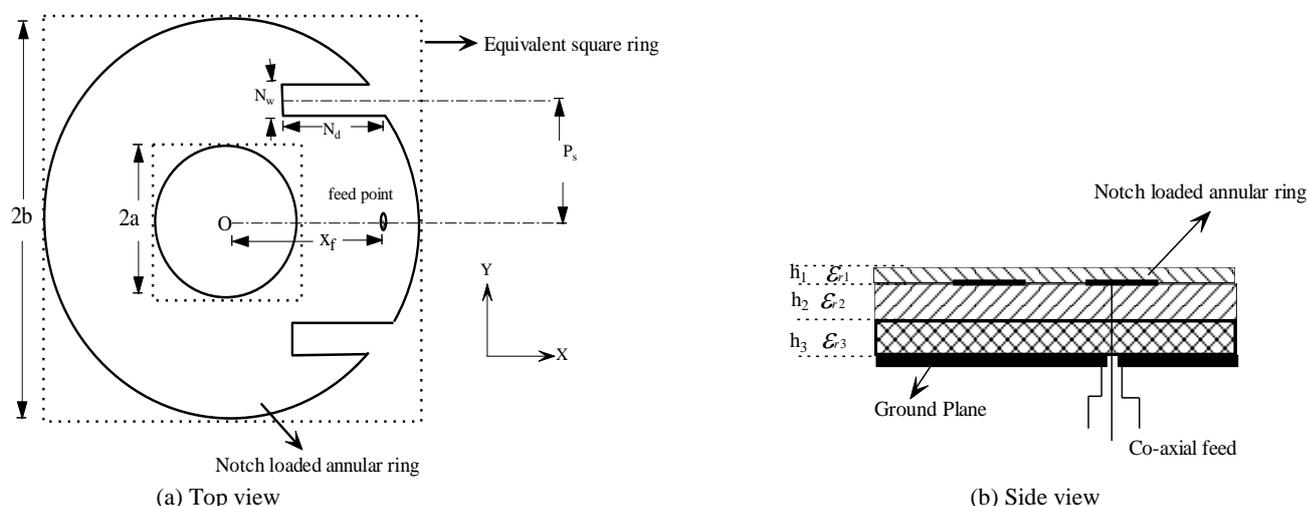
**Fig.1** Configuration of proposed antenna
