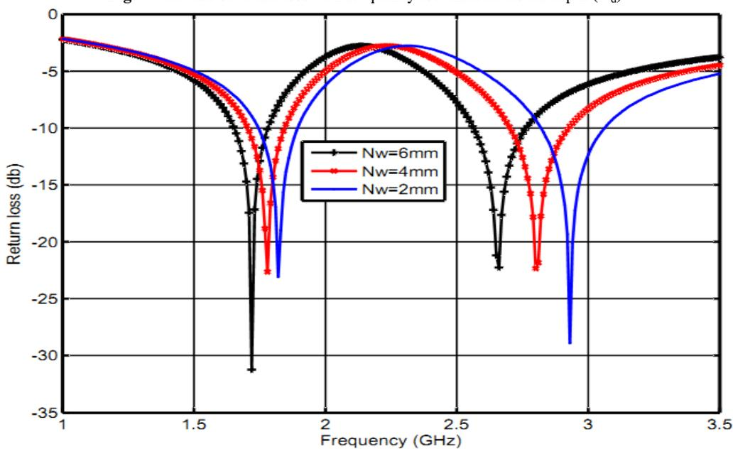
Fig.5 Variation of return loss with frequency for different notch width ( $N_w$ )
