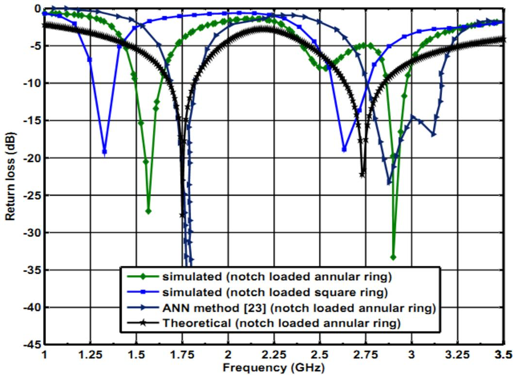
Fig.7 Comparative results of return loss with frequency of the ARMA for proposed, simulated and ANN method
