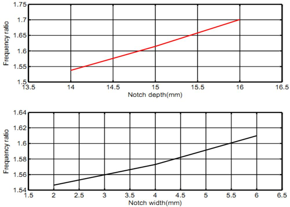
Fig.6 Variation of frequency ratio with different notch depth ( $N_d$ ) and notch width ( $N_w$ )
