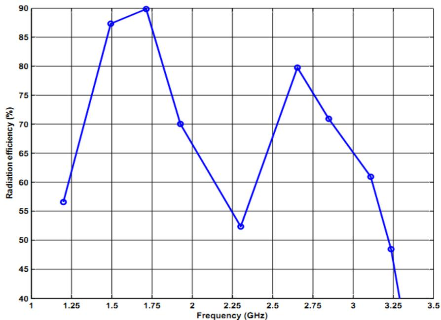
Fig. 11 Radiation efficiency of the proposed antenna
