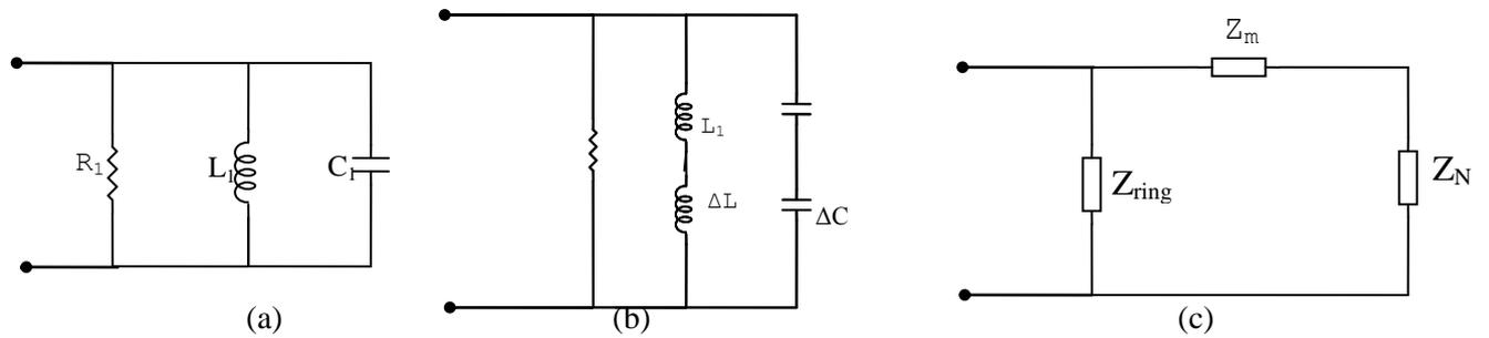
**Fig. 2** Equivalent circuit of (a) ARMA (b) notched ARMA (c) Modified notched ARMA
