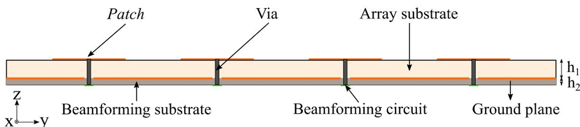
Fig. 11. The cross section of the array topology.
