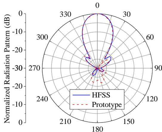
Fig. 18. Experimental and simulated normalized radiation patterns.
