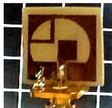
Fig.8. Fabricated prototype of the proposed antenna.
