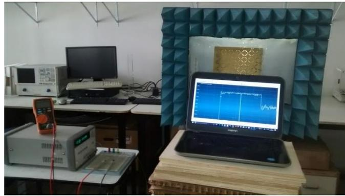
Fig. 17. Wi-Fi signal strength response displayed on notebook, y polarization..
