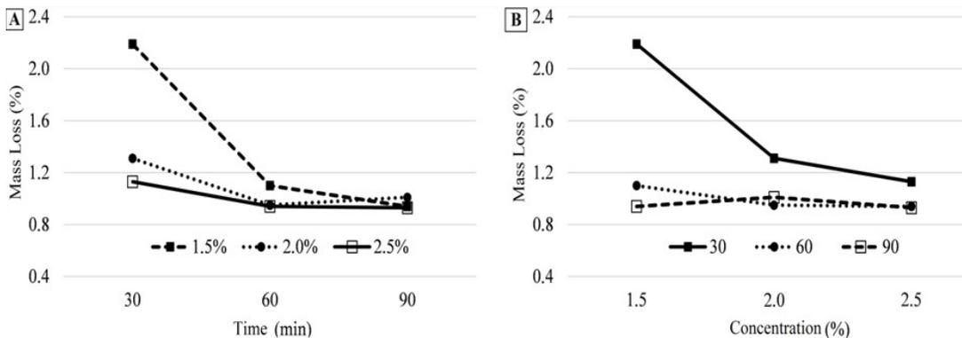
**Figure 2.** Interaction between time (A) and CCB concentration (B) in the urograndis wood mass loss in the presence of *Trametes versicolor*.
