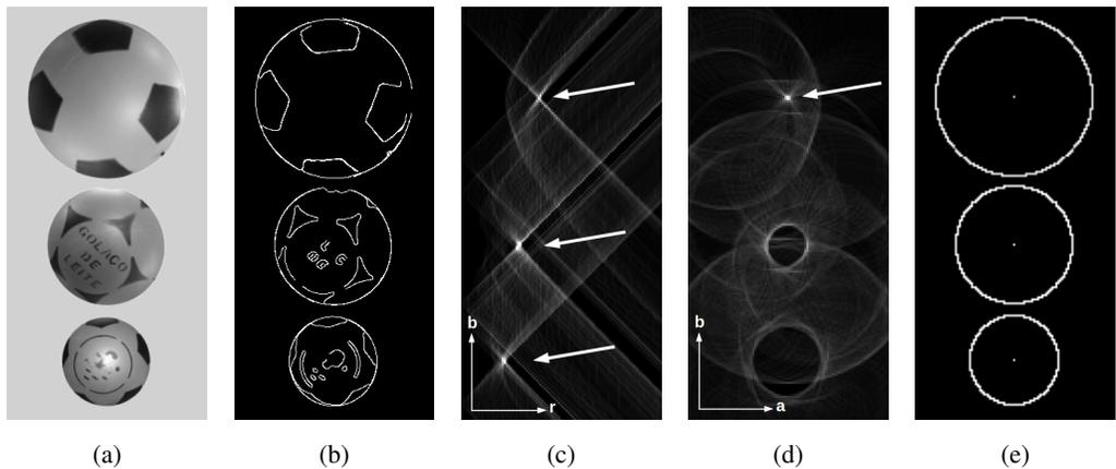
Figure 2: Steps for detecting circles using the Hough transform. (a) The image is smoothed using Gaussian filter. (b) Edges are detected using Canny filter. (c-d) Accumulated votes in 3D parameter space are shown in planar sections with arrows highlighting local maximums. (e) The parameters indicated by the local maximums are used to reconstruct the circles.
