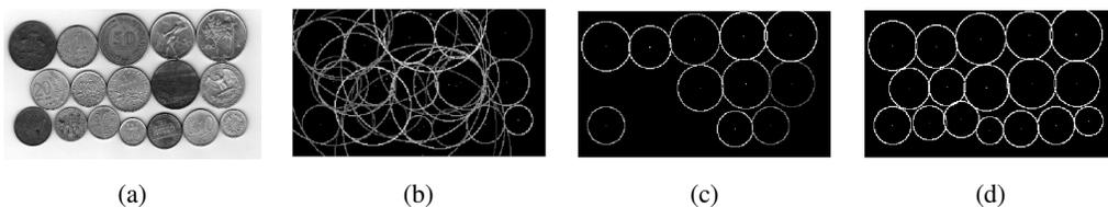
Figure 4: Comparison on the multiple circles detection. (a) Real image with 17 coins. (b) Using standard voting and threshold 50, some false circles are detected. (c) Using threshold 80 some true circles are removed. (d) All true circles are detected without the appearance of false circles using the proposed voting process.
