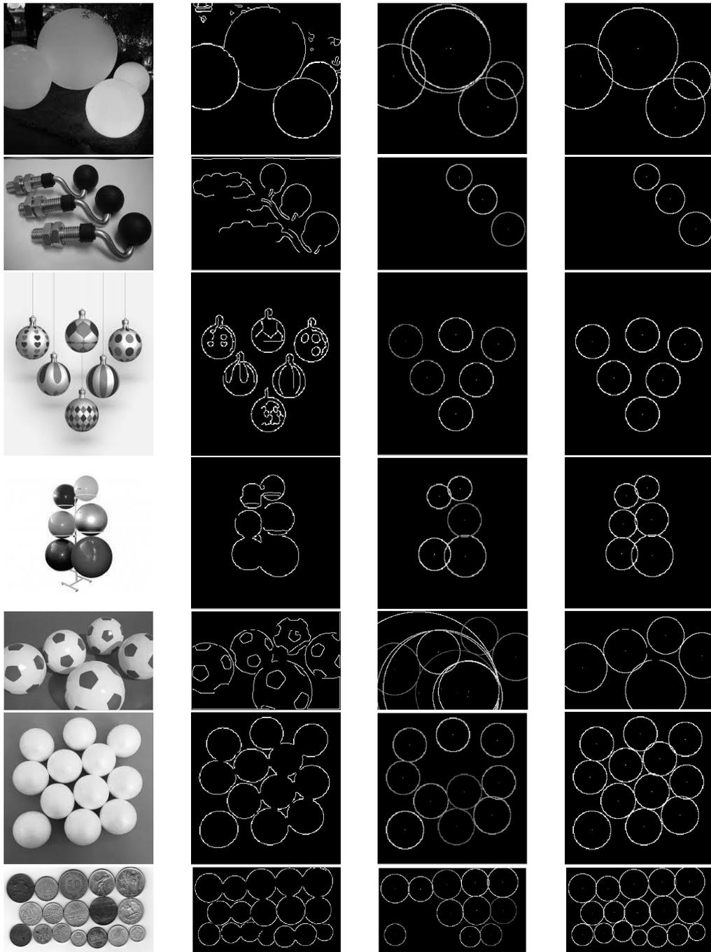
Figure 6: Comparison of results. The first column shows a set of 7 real images. In the second column, the edge points are detected. In the third column, the circles detected with the standard direct voting process. In the last column, the circles detected with our voting process inversely proportional to the radius.
