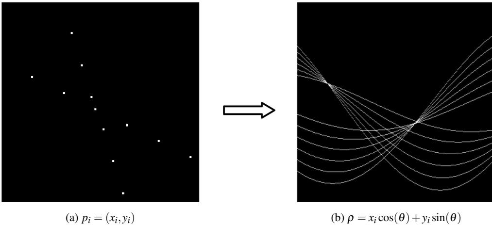
Figure 1: Mapping from a set of points in the image domain to the parameters domain. In (a) we have 12 points along two lines and, in (b), each point is represented by a curve in the parameter space. Notice that each set of 6 curves defines an intersection point. The coordinates of these points of intersection are the parameters of the curves that best fit the points in the image
