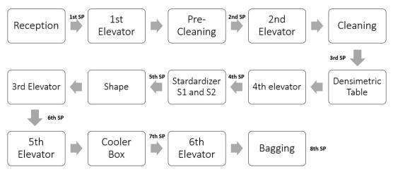
Figure 1. Flowchart of the stages of the processing of soybean seeds and the Sampling Points (PA) in the Seed Processing Unit of the company CIASEEDS in Correntina, BA.
