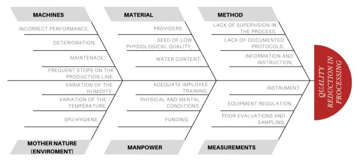
Figure 2. Diagram of Cause and Effect (6 M's) of the processing of soybean seeds. Source: Research data.
