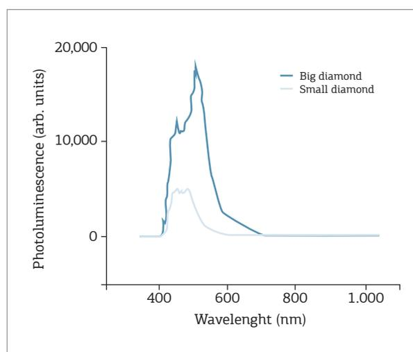
Figure 9. Photoluminescence of both diamonds.
