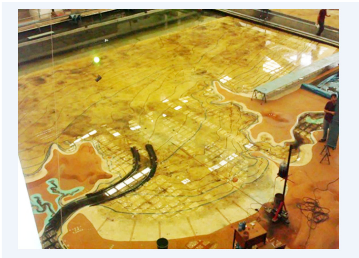
Figure 3. Physical model of the Bay and Estuary of Santos and São Vicente with Gireli et al. (2010) proposed jetties. Source: Gireli et al. (2010).
