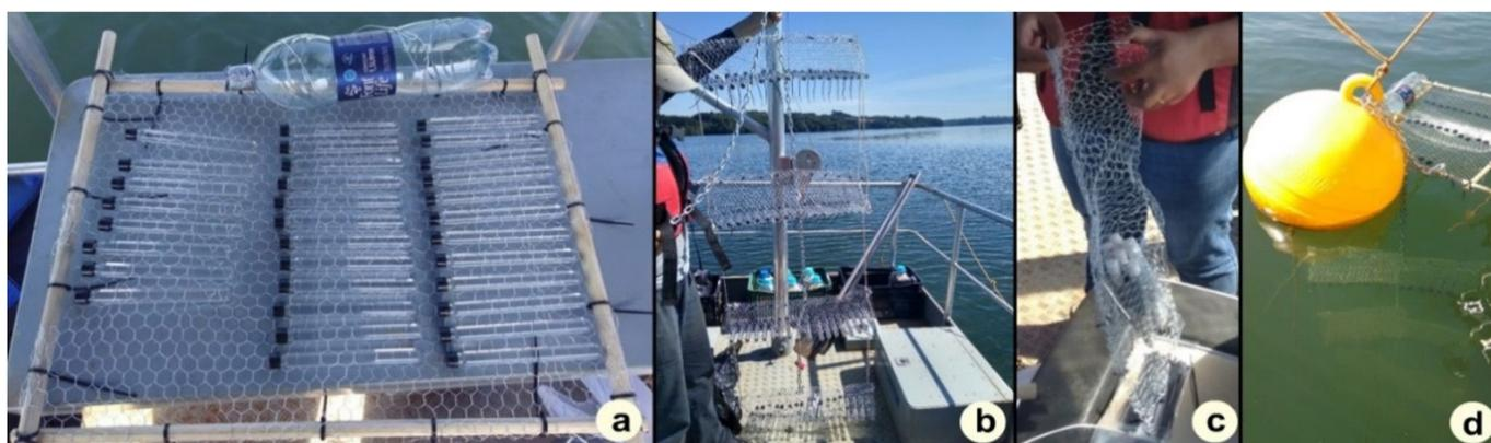
**Figure 2.** Sample fixing structure for photodegradation in different depths: photodegradation sets (a) on the surface; (b) every 0.5 m; (c) dark control (d) start of incubation in the reservoir (Souza et al., 2019).
