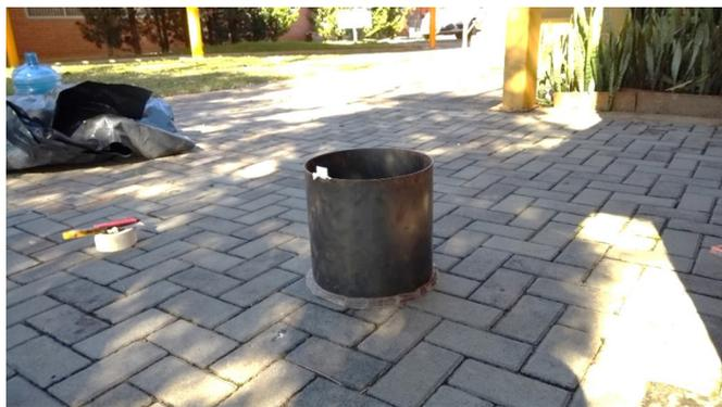
**Figure 3.** Example of the 0.30 m-diameter infiltrometer ring placed over the ICP surface.
