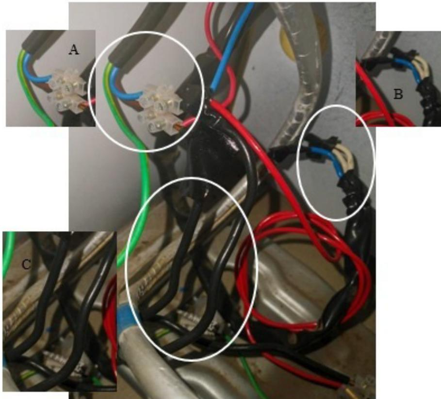
**Figure 7.** Connection of the refrigerator and compressor cables where it was interrupted to change the compressor command to the temperature controller; (A) wires that conduct the energy to the compressor. (B) wires from the refrigerator's internal equipment; (C) phase and neutral wires that feed the temperature controller.
