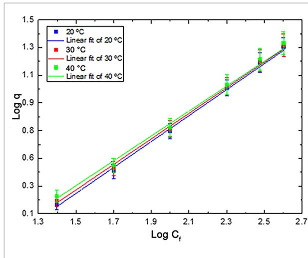
Figure 5 - Adsorption isotherm of *R. opacus* onto apatite surface. The data were fitted with *Freundlich* model (Temperature: 20°, 30°, 40° C).
