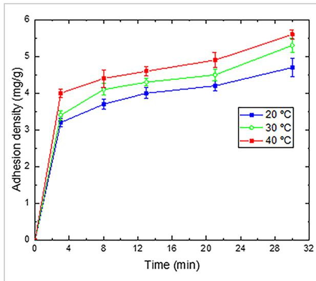
Figure 6 - Effects of time and temperature on the adsorption density: pH 7 and cell concentration of 100 mg/L (Temperature: 20, 30 and 40° C).
