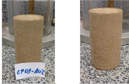
Figure 2 - Triaxial test specimens with 10% cement content.
