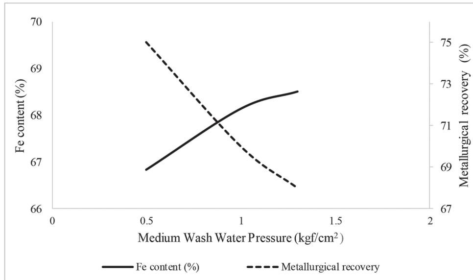
Figure 6 - Magnetic concentration test 6 varying the average water pressure.
