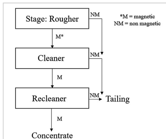
Figure 1 - Magnetic concentration flowchart.
