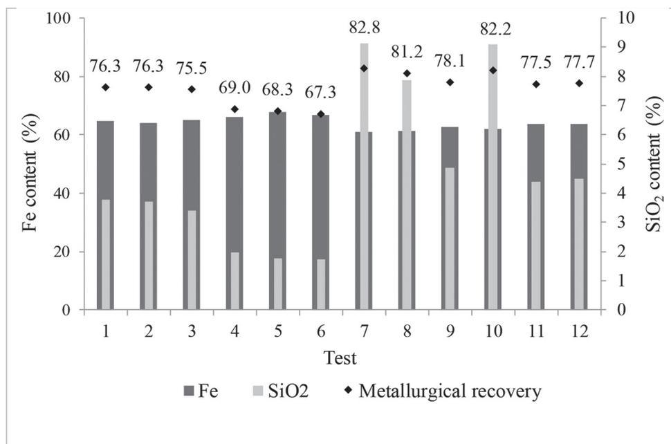
Figure 5 - Magnetic concentration tests.
