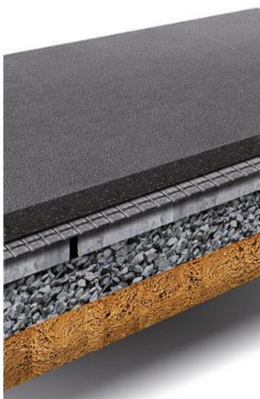
Figure 2 – Cross-section using the geogrid. Source: Huesker, 2022.
