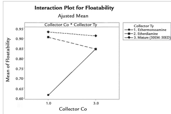
Figure 4 - Plot of the adjusted means interaction for floatability.
