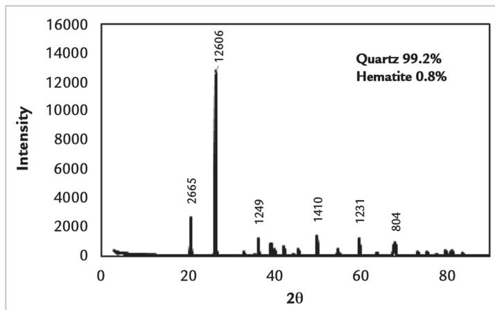
Figure 1 - X-ray diffraction of quartz.
