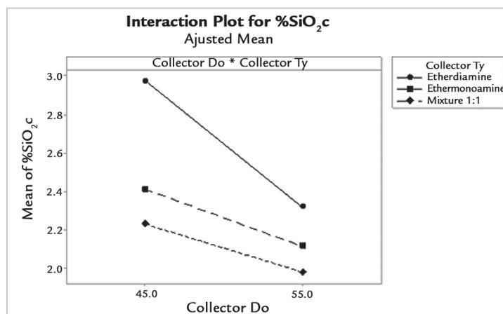
Figure 7 - Plot of main effects of the adjusted means for %SiO<sub>2</sub> in concentrate.
