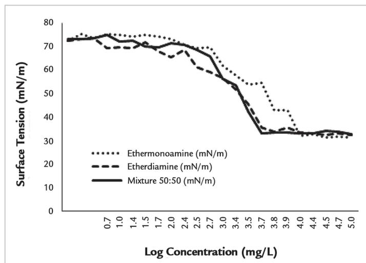
Figure 2 - Surface tension versus concentration of etheramines and their mixtures.
