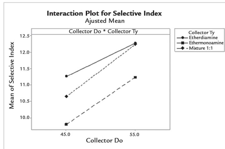
Figure 9 - Plot of main effects of the adjusted means for Selective Index.
