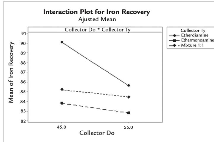
Figure 8 - Plot of main effects of the adjusted means for iron recovery.
