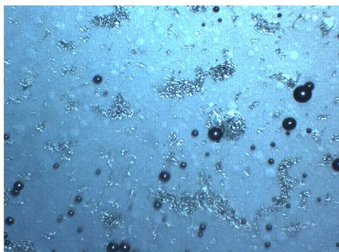
Figure 1 - Signals of destabilization of explosive emulsion through appearance of ammonium nitrate crystals. Note that there are some dark spheres. They are entrapped air bubbles, not crystals.
