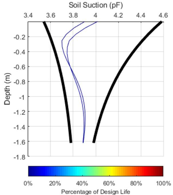
Figure 11. The estimated initial suction profiles (time = 2 months) for TX 48-1068 section.
