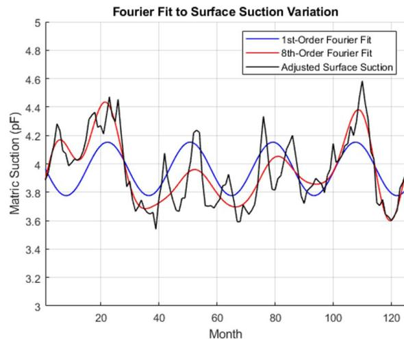
**Figure 9.** 1<sup>st</sup> and 8<sup>th</sup> order Fourier fit to the surface suction data for the TX 48-1068 section for the date range 3/1987 to 9/1997.
