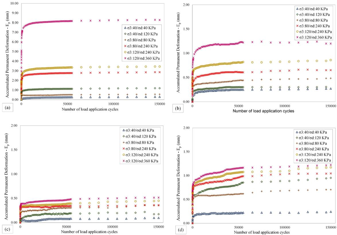
Figure 4. Accumulated permanent deformation of (a) standard energy, (b) intermediate energy, (c) modified energy and (d) undisturbed from top layer.
