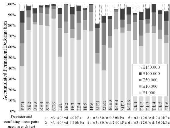
**Figure 5.** Part of accumulated permanent deformation as cycles increase.
