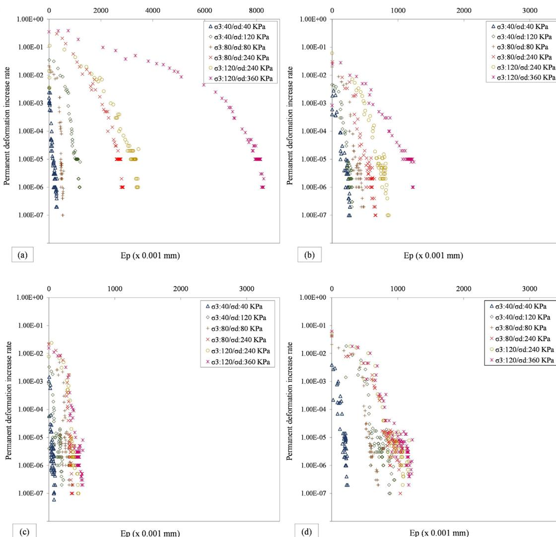
**Figure 6.** Shakedown occurrence research according to Dawson & Wellner (1999) of the (a) standard energy, (b) intermediate energy, (c) modified energy and (d) undisturbed of top layer.
