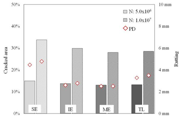
**Figure 7.** Comparison of four structural performance in the face of permanent deformation (rutting) and fatigue (cracked area) submitted to two  $N$ .
