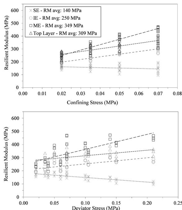
**Figure 2.** Comparison between deviator stress and confining stress for the four resilient modulus conditions.
