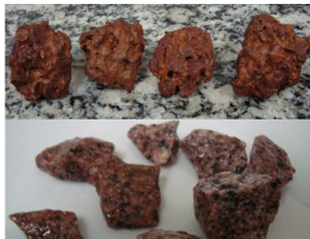
Figure 4. Visual comparison between the porosities of the Acre laterite pores (above) and the crushed granite (below).
