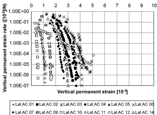
Figure 8. Vertical permanent strain rate versus vertical permanent strains of the Acre laterite of this study.
