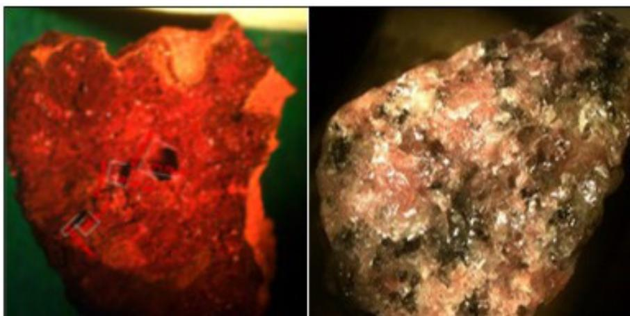
**Figure 5.** A microscopic image (magnification factor of 6.5) of (a) a sample of the Acre laterite gravel evaluated in this study and (b) a sample of crushed granite for comparison.
