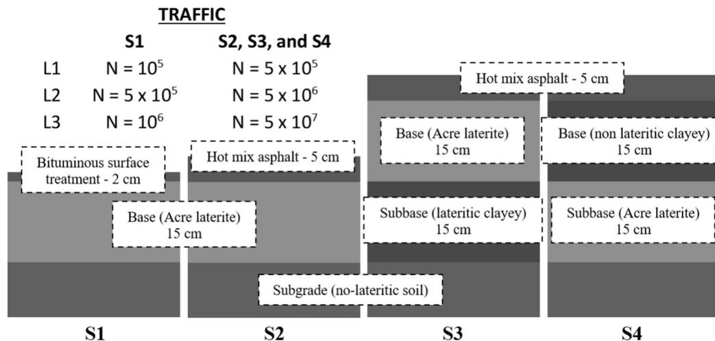
Figure 6. Information about the four sections analyzed in this study.
