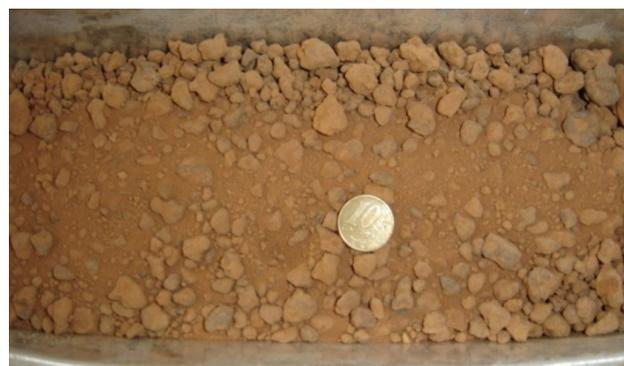
Figure 3. Illustration of the Acre laterite gravel evaluated in this study.
