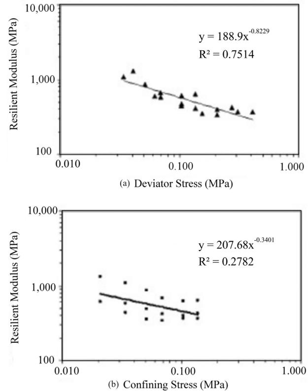
**Figure 9.** Relationship between the *RM* results for the Acre laterite gravel evaluated in this study and the (a) deviator stress and (b) confining stress.
