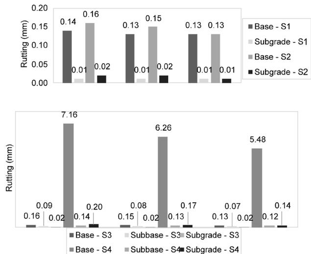
**Figure 10.** Rutting predicted from MeDiNa simulations for different traffic levels and pavement structures using the Acre laterite gravel in the composition of the base or subbase layers.
