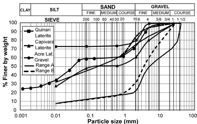
Figure 2. Gradation distributions of three Acre laterite gravels, including the one evaluated in this study, and two gradation envelopes from the Brazilian standard DNIT 098 (DNIT, 2007).
