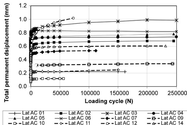
Figure 7. Total permanent displacements for the Acre laterite of this study subjected to various stress states.
