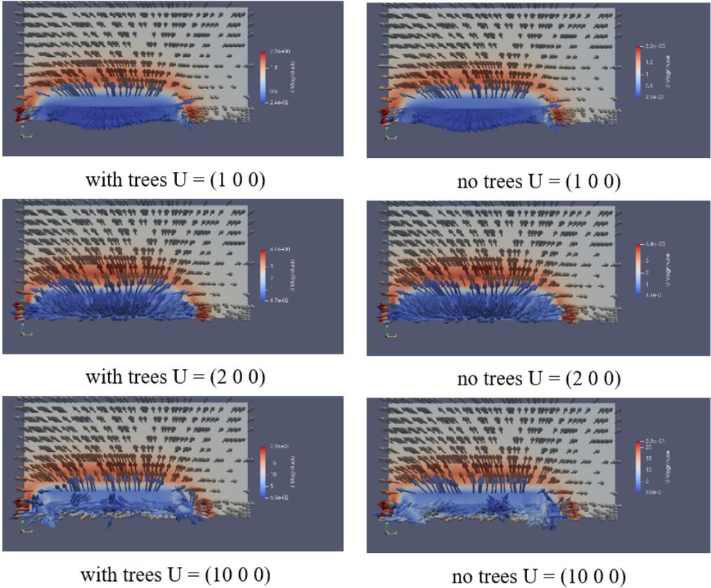
Figure 3: Velocity profiles for perpendicular wind incidence, with and without trees.
