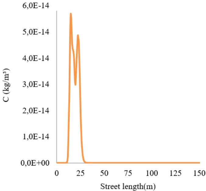
Figure 7: Pollutant concentration, with initial wind velocity 10 m/s with trees, perpendicular to the street axis -  $U = (0,10,0)$ .
