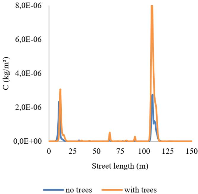
Figure 4: Pollutant concentration for initial wind velocity 10 m/s, perpendicular to the street main axis,  $U = (0,10,0)$ .
