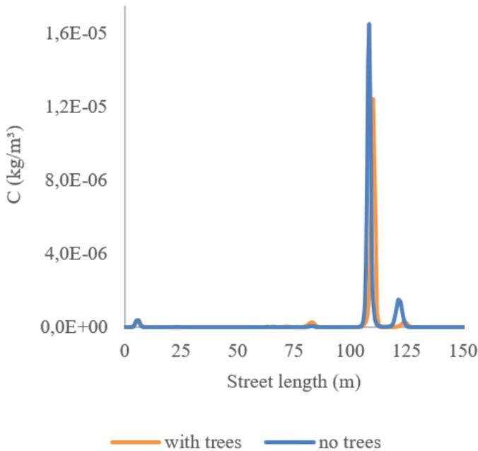
Figure 9: Pollutant concentration, with initial wind velocity 10 m/s with trees, perpendicular to the street axis -  $U = (0,10,0)$ .
