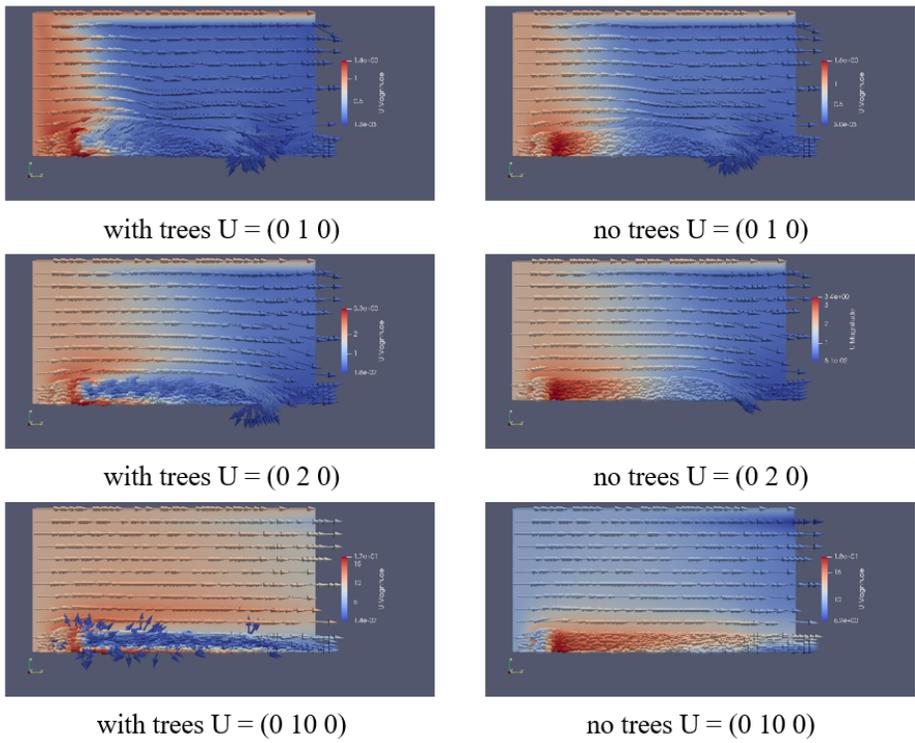
Figure 5: Velocity profile, with wind field parallel to the street axis, with and without trees.
