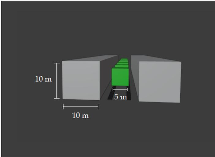
Figure 1: Urban canyon geometry used on simulations.
