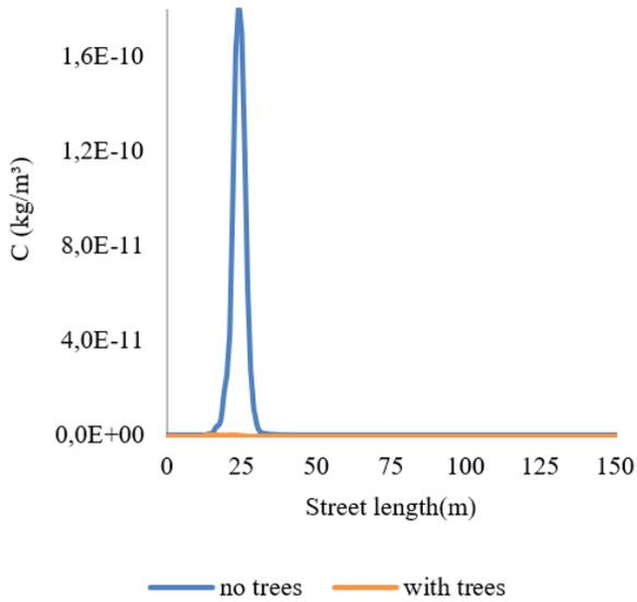
Figure 6: Pollutant concentration, for wind initial velocity 10 m/s, perpendicular to the street main axis -  $U = (0,10,0)$ .
