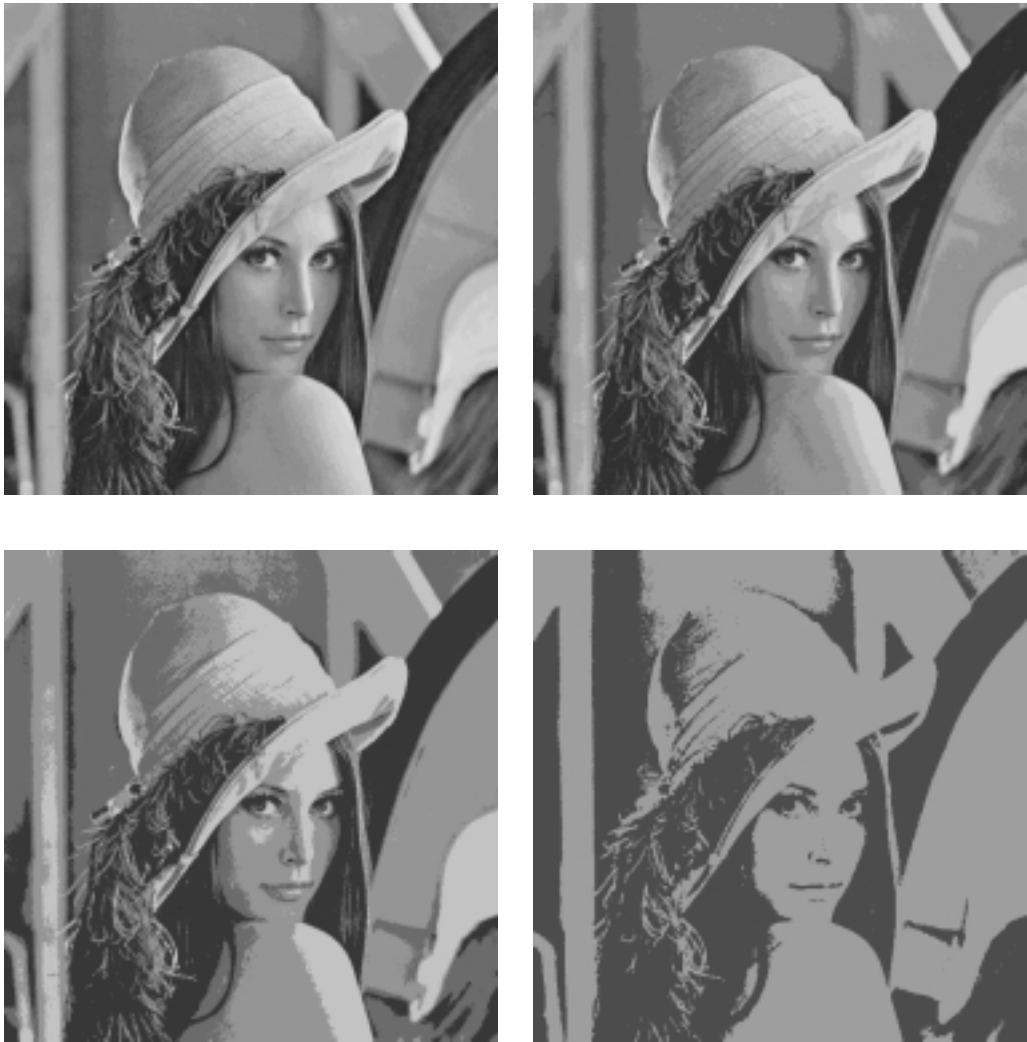
Fig. 2 – Lena image quantized to 16, 8, 4 and 2 bits/pixel and distortion measure d(x, y) = |x - y|^2 .
