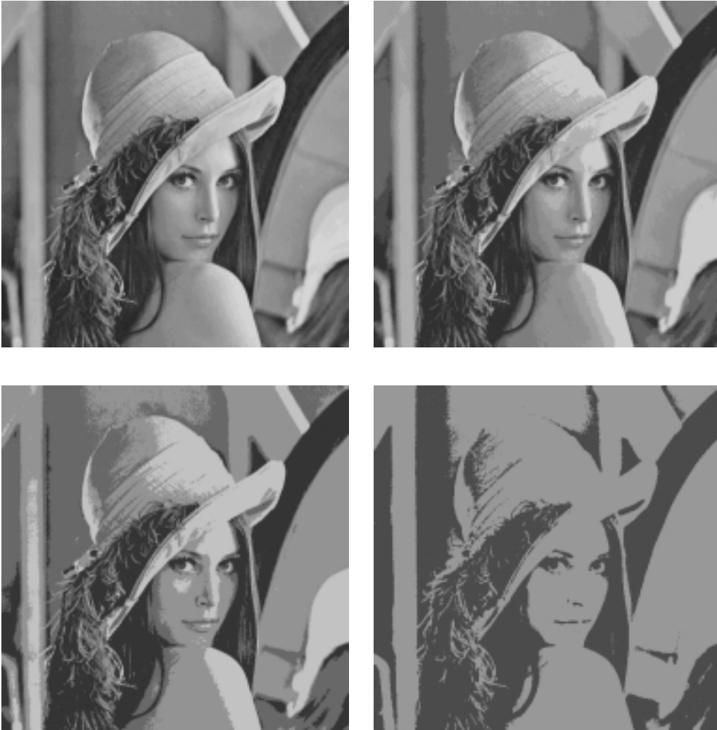
Fig. 1 – Lena image quantized to 16, 8, 4 and 2 bits/pixel and distortion measure d(x, y) = |x - y| .
