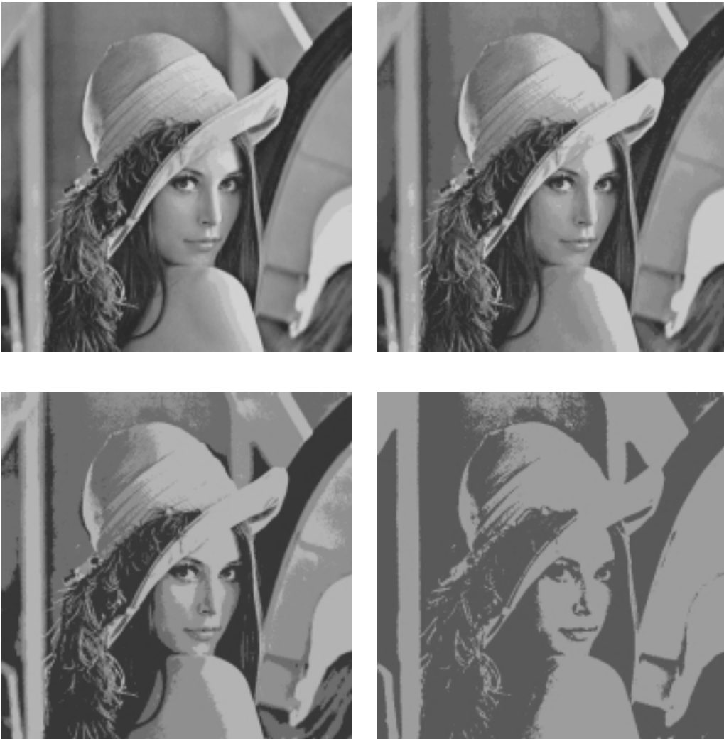
Fig. 5 – Lena image quantized to 16, 8, 4 and 2 bits/pixel and using the median cut algorithm.
