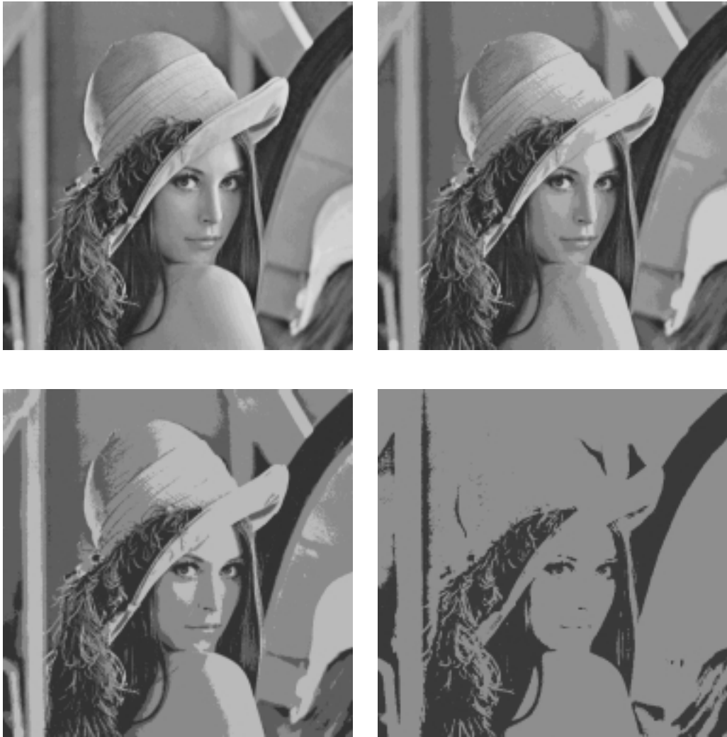
Fig. 4 – Lena image quantized to 16, 8, 4 and 2 bits/pixel and distortion measure d(x, y) = |\log(x) - \log(y)|^2 .
