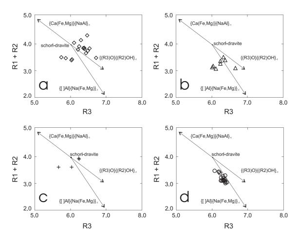
Fig. 5 – Representation of tourmaline compositions in the R1 + R2 vs. R3 diagram (R1, R2 and R3 calculated after Yavuz 1997). Tourmalines from: (a) metachert – Tapera Grande and Quartzito; (b) tourmalinite – Tapera Grande; (c) quartz vein – Tapera Grande, and (d) quartz vein – Quartzito.
