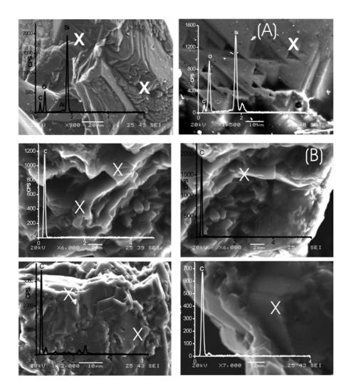
Fig. 5 – (A) SEM images and EDS spectrum of grains composed exclusively of SiO<sub>2</sub> with dissolution structures. (a) corrosion structures and negative trygons; (b) negative trygons. The trygons were originated by dissolution. X = analized points. (B) SEM images and EDS spectrum of grains composed exclusively of carbon identified in heavy mineral concentrates from the intrusive rocks. X = analized points.
