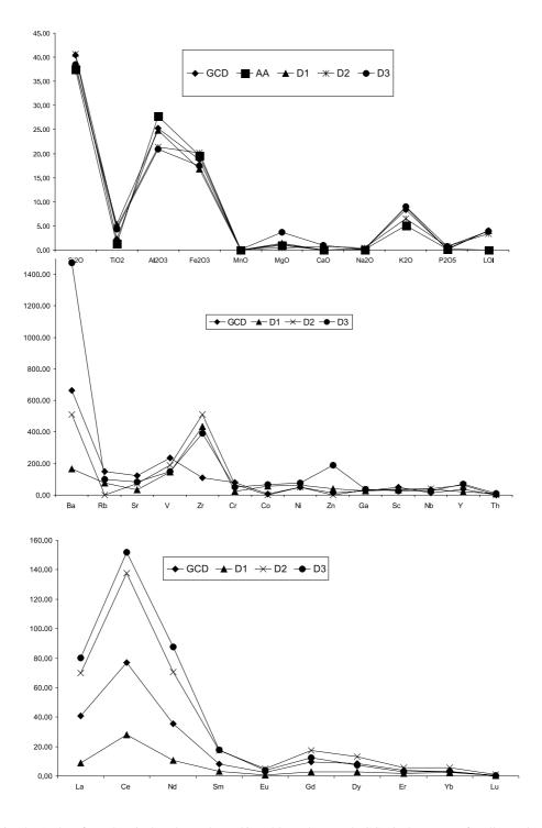
Fig. 4 - A plot of geochemical analyses showed in Table I. The sample GCD is the average for all samples from Chapada Diamantina – BA. Major elements (wt %), trace and REE elements (in ppm). Observe that the elements behavior of the Chapada Diamantina samples is similar to the elements behavior of the hematitic philite from Diamantina – MG.
