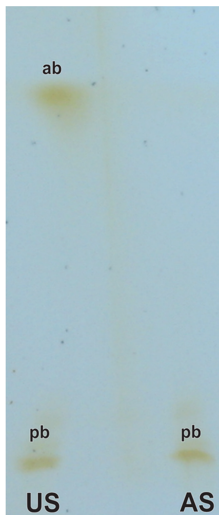
Figure 5 - Thin layer chromatography (TLC) of terpenoids and other volatile compounds from extracts of bark powder of the underground stem (US) and aerial stem (AS) of Tontelea micrantha . ab: more apolar band; pb: more polar band.
