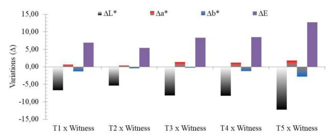
**Figure 4.** Variations between the values of the colorimetric parameters of the wood samples of *Gmelina arborea* after the application of the treatments in relation to the control wood.
