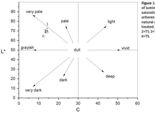
Figure 3. Diagram of luminosity (L\*) x saturation (C) of Gmelina arborea samples in natural condition and treated. Note: 1=Control; 2=T1; 3=T2; 4=T3; 5=T4; 6=T5.
