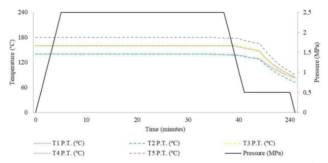
**Figure 1.** Diagram of the thermomechanical densification process with the temperatures of the hydraulic press (P.T. = Press temperature).
