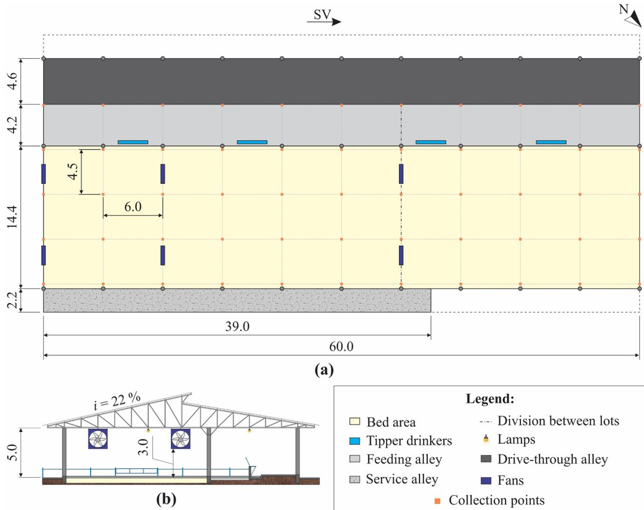
**Figure 1. Schematic representation of the Compost-Bedded Pack Barn facility where the experimental data were collected: (a) floor plan with collection points and (b) cross-sectional. \*SV – sense of ventilation;  $i$  – roof slope; N – North indication; dimensions in meters (m).**
