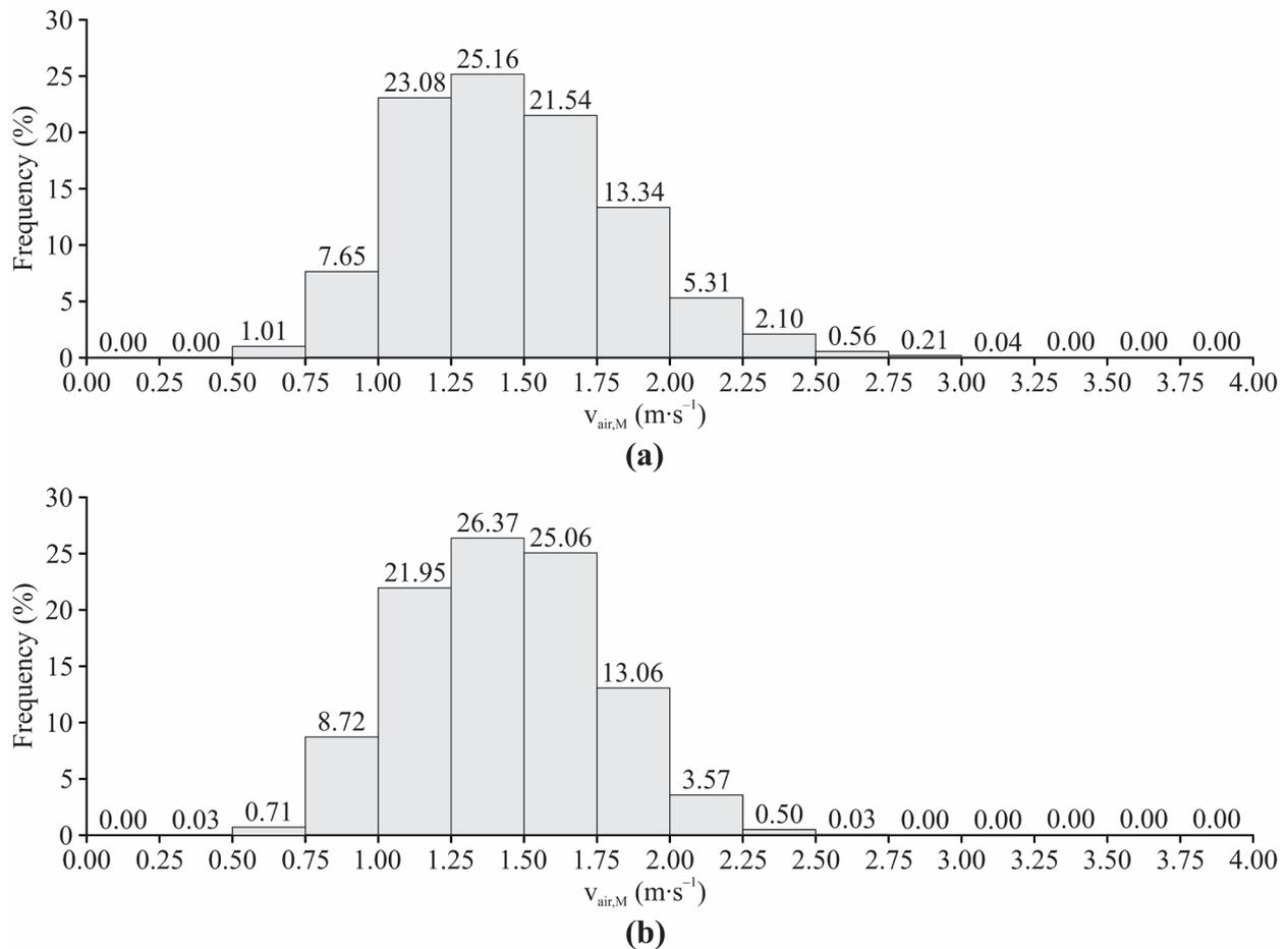
**Figure 3. Frequency distribution of air velocity at the 1.5 m height ( $v_{air,M}$  in  $m \cdot s^{-1}$ ): (a) morning and (b) afternoon periods.**
