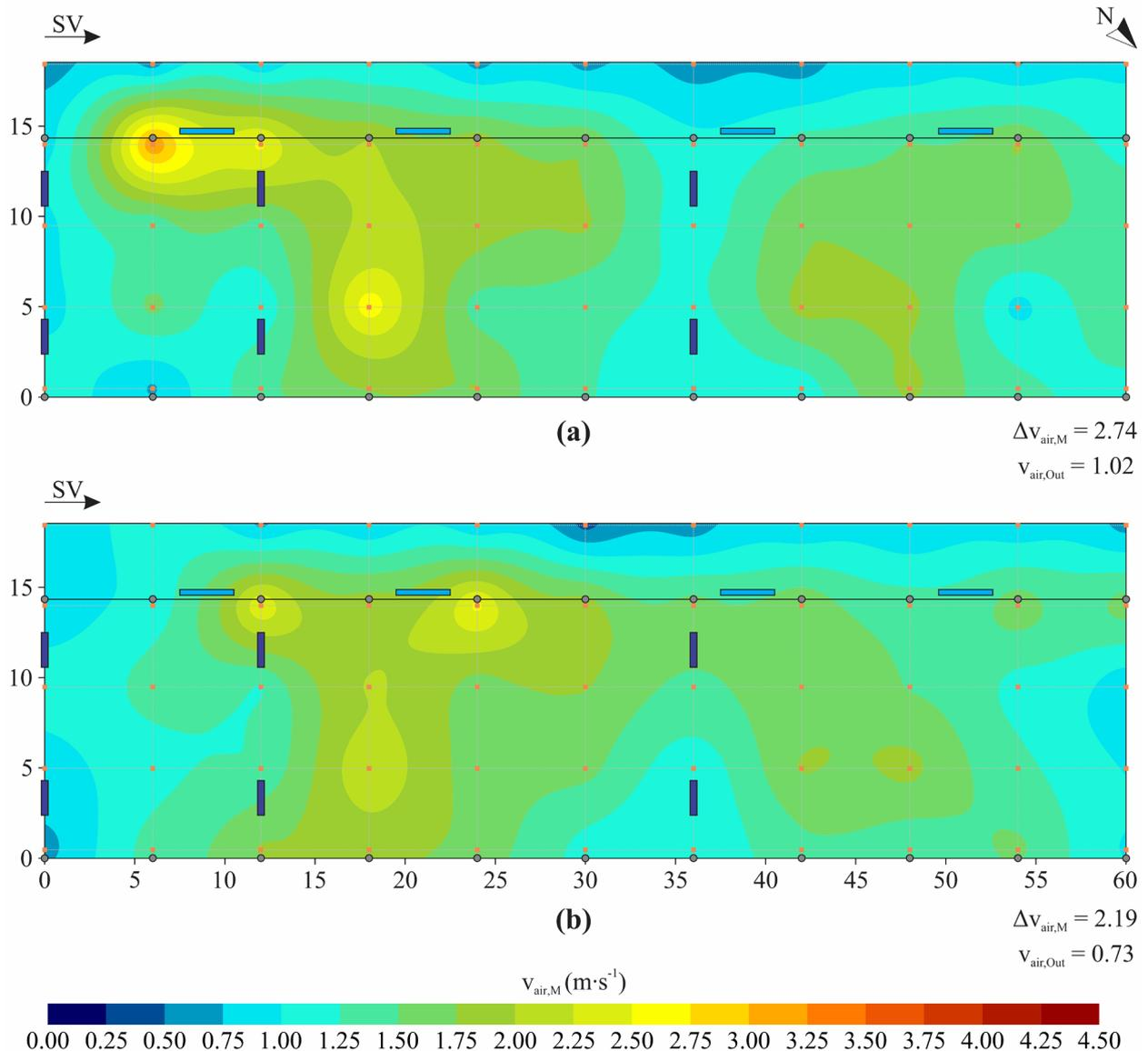
**Figure 2. Spatial distribution of air velocity at the 1.5 m height ( $v_{\text{air},M}$  in  $\text{m}\cdot\text{s}^{-1}$ ): (a) morning and (b) afternoon periods. \*SV – sense of ventilation;  $\Delta v_{\text{air},M}$  – air velocity variation at the 1.5 m height;  $v_{\text{air},\text{Out}}$  – average air velocity outside the facility; N – North indication; dimensions in meters (m).**
