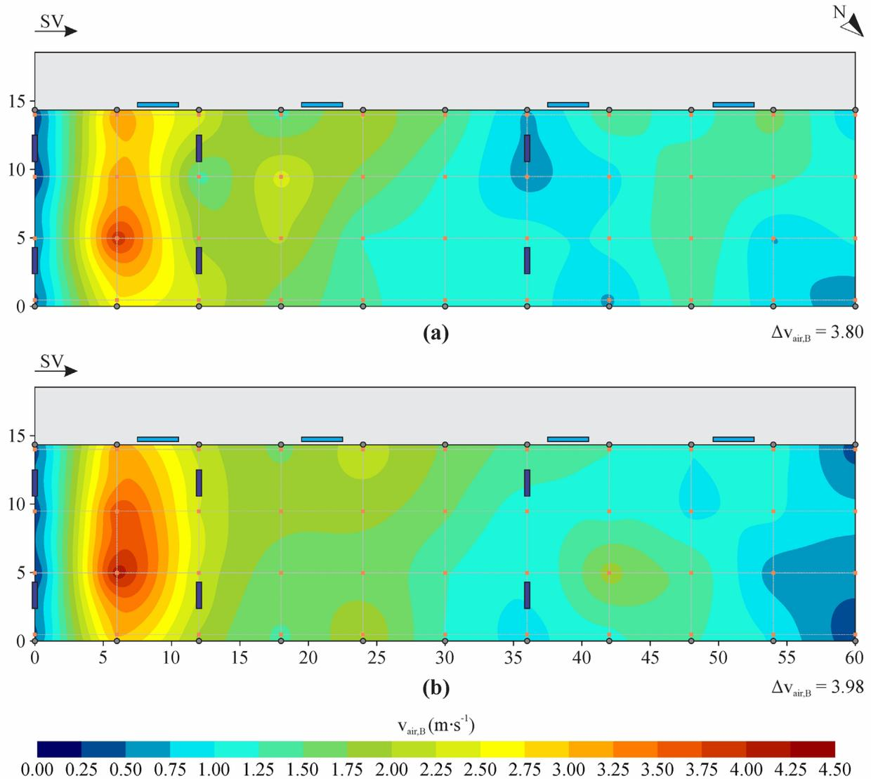
**Figure 4. Spatial distribution of air velocity at bedding level ( $v_{air,B}$ , in  $m \cdot s^{-1}$ ): (a) morning and (b) afternoon periods. \*SV – sense of ventilation;  $\Delta v_{air,B}$  – air velocity variation at bedding level; N – North indication; dimensions in meters (m).**
