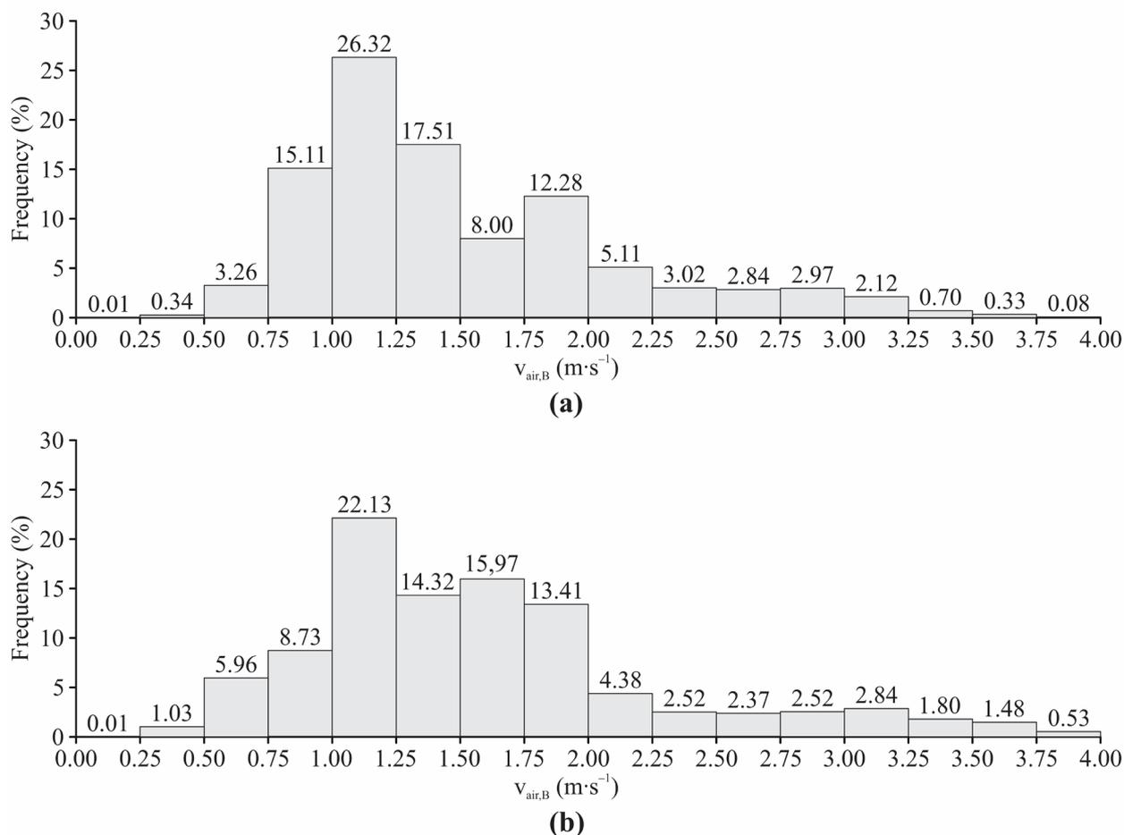
**Figure 5. Frequency distribution of air velocity at bedding level ( $v_{air,B}$ , in  $m \cdot s^{-1}$ ): (a) morning and (b) afternoon periods.**
