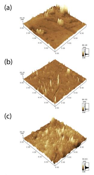
**Figure 3.** Nanometer roughness profile of titanium surfaces. (a) Polished surface profile. (b) CAP-treated surface profile. (c) Low pressure plasma nitrided surface.
