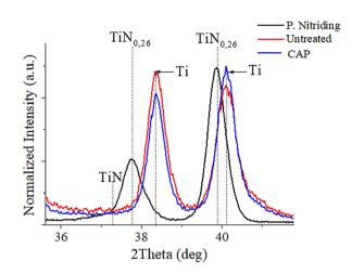
**Figure 4.** Diffractogram of titanium surfaces at a 2° Theta grazing angle.
