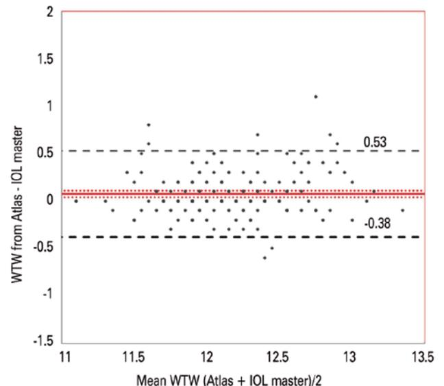
**Figure 3.** Bland-Altman Plot of white-to-white distance values measured with the Atlas topographer and IOL Master. Limits of agreement for the Atlas topographer and IOL Master fell between -0.38 to +0.53 mm with a relatively uniform distribution. Red line = bias; red dot lines = 95% confidence interval of the bias; dashed lines = 95% limits of agreement.
